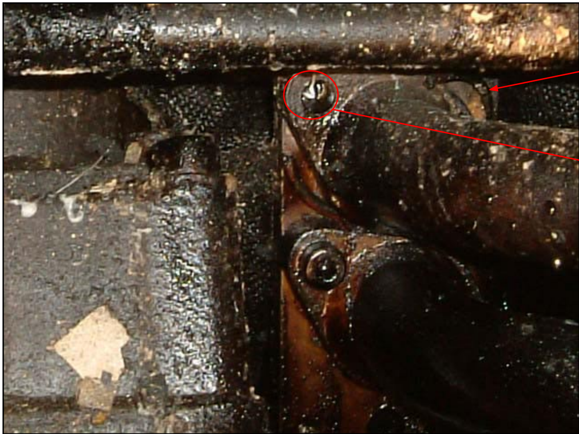
Fuel pipe flange and "O" ring seal
