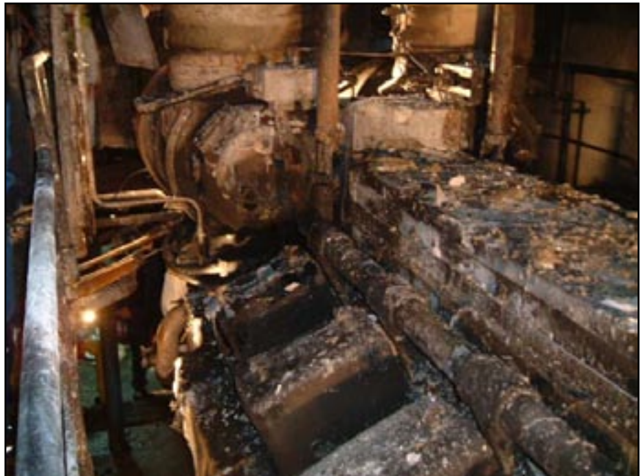
Damaged rocker covers, camshaft and crankcase doors
