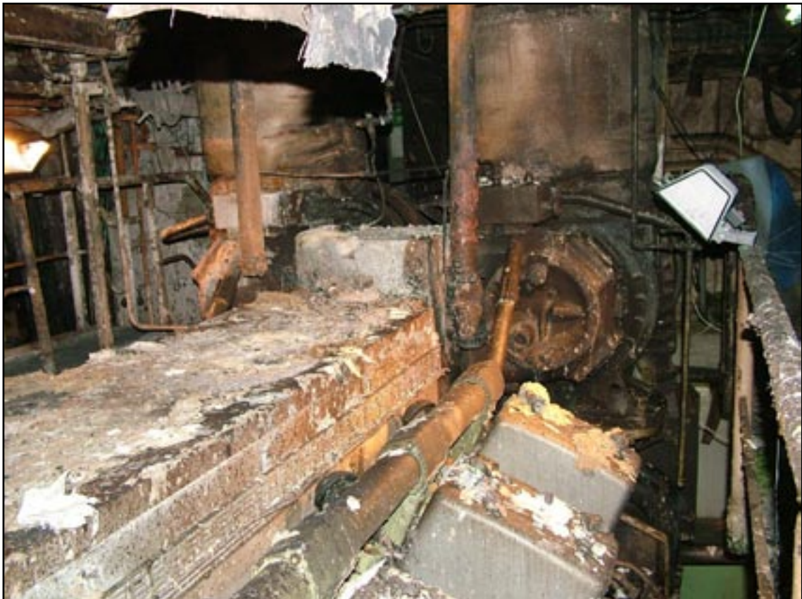
Fire damaged turbo chargers
