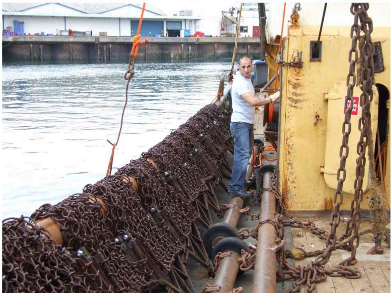
With turns of the "tipping" rope placed around the whipping drum, the latter is used to raise the "hook end" of the "tipping" rope....
