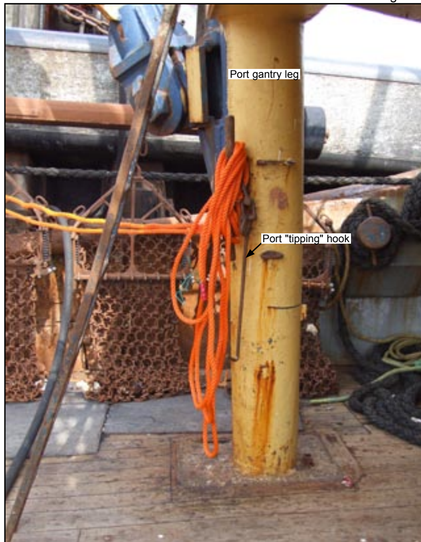
Port gantry leg and stowed port "tipping" hook
