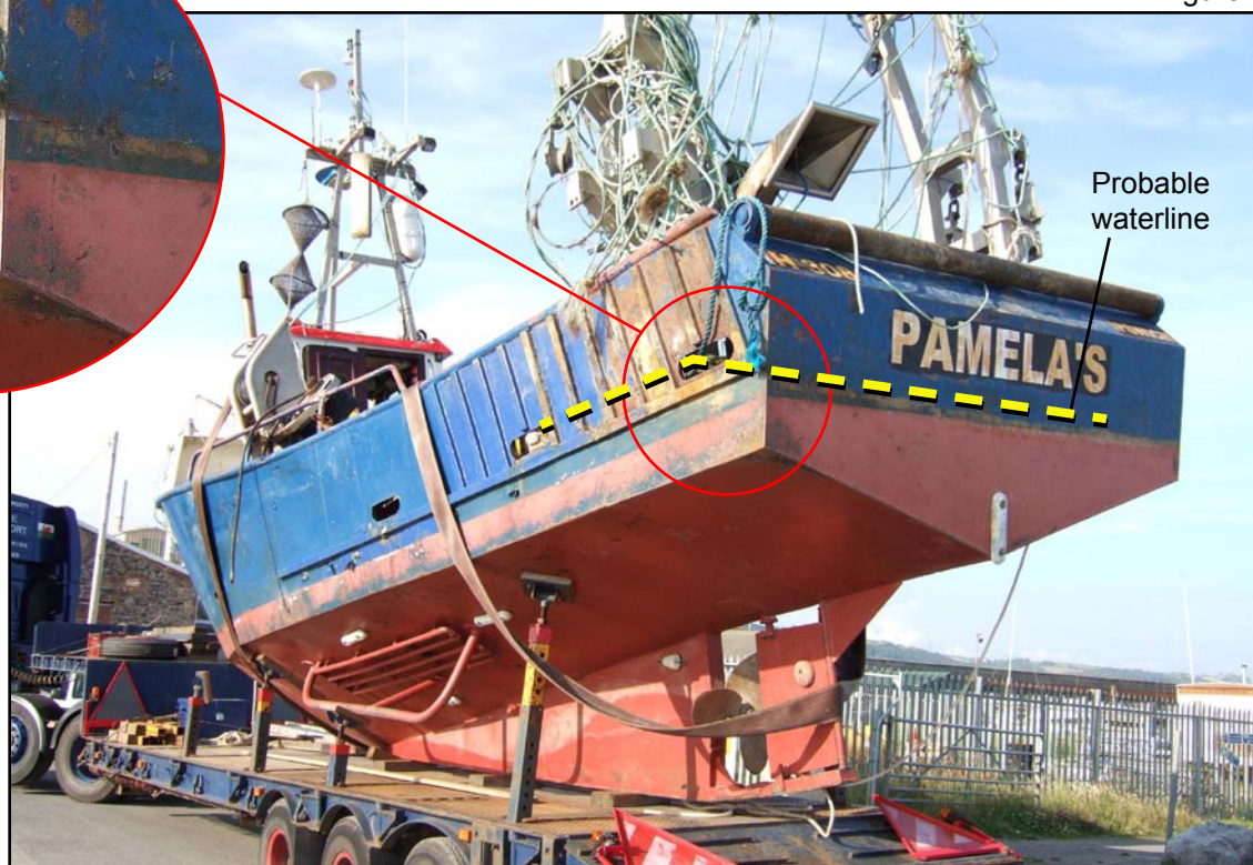
Probable waterline level as vessel left its moorings on 17 June 2006
