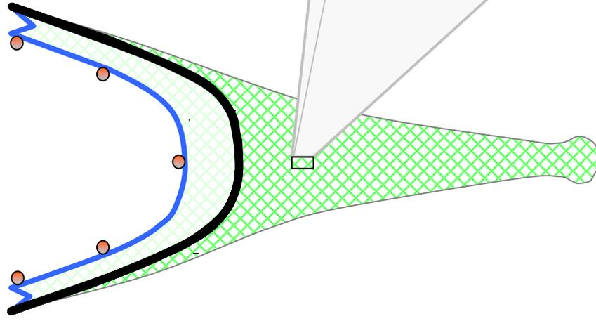
Position of stone trap in the belly of the net. At least 10 ft behind the fishing line to save distorting the net. More than one trap can be fitted, one behind the other with at least 10 feet between them.
