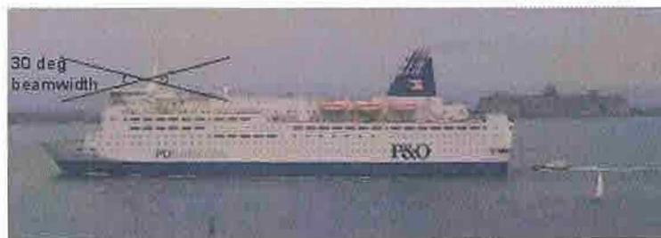
Figure 7 Diagram showing the elevation beamwidth of the S-Band radar overlaid on a photo of the Pride of Bilbao
