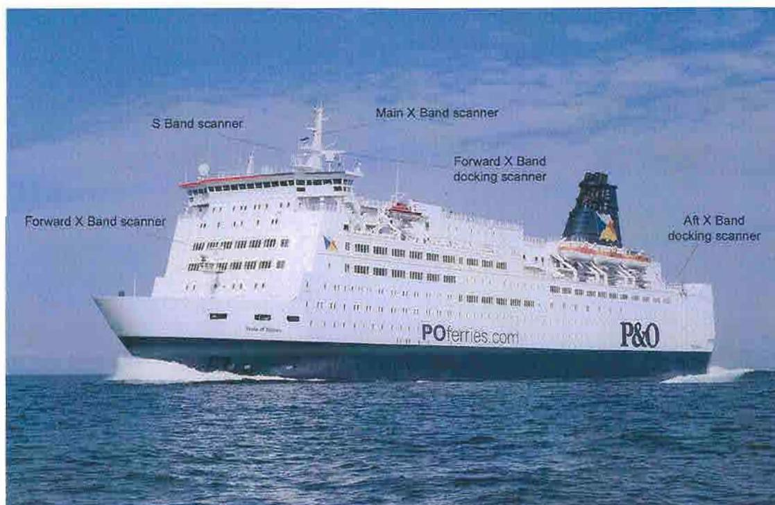
Figure 6 Photograph of the Pride of Bilbao showing the location of its radar scanners.
