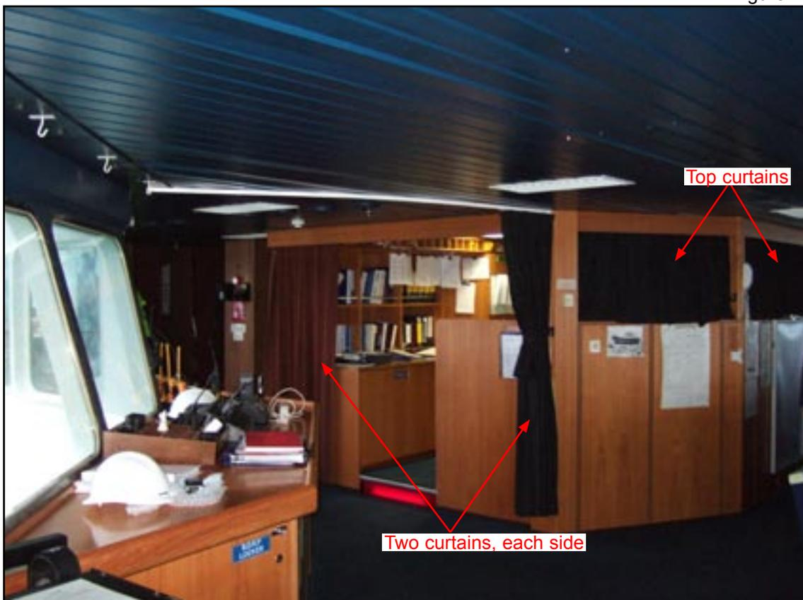
Starboard side curtains, and port side were in open position as shown
