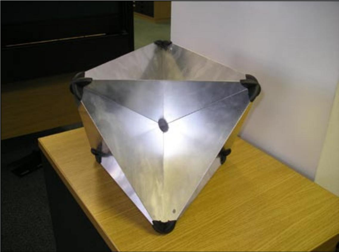
Octrahedral type radar reflector ("catch rain" position)
