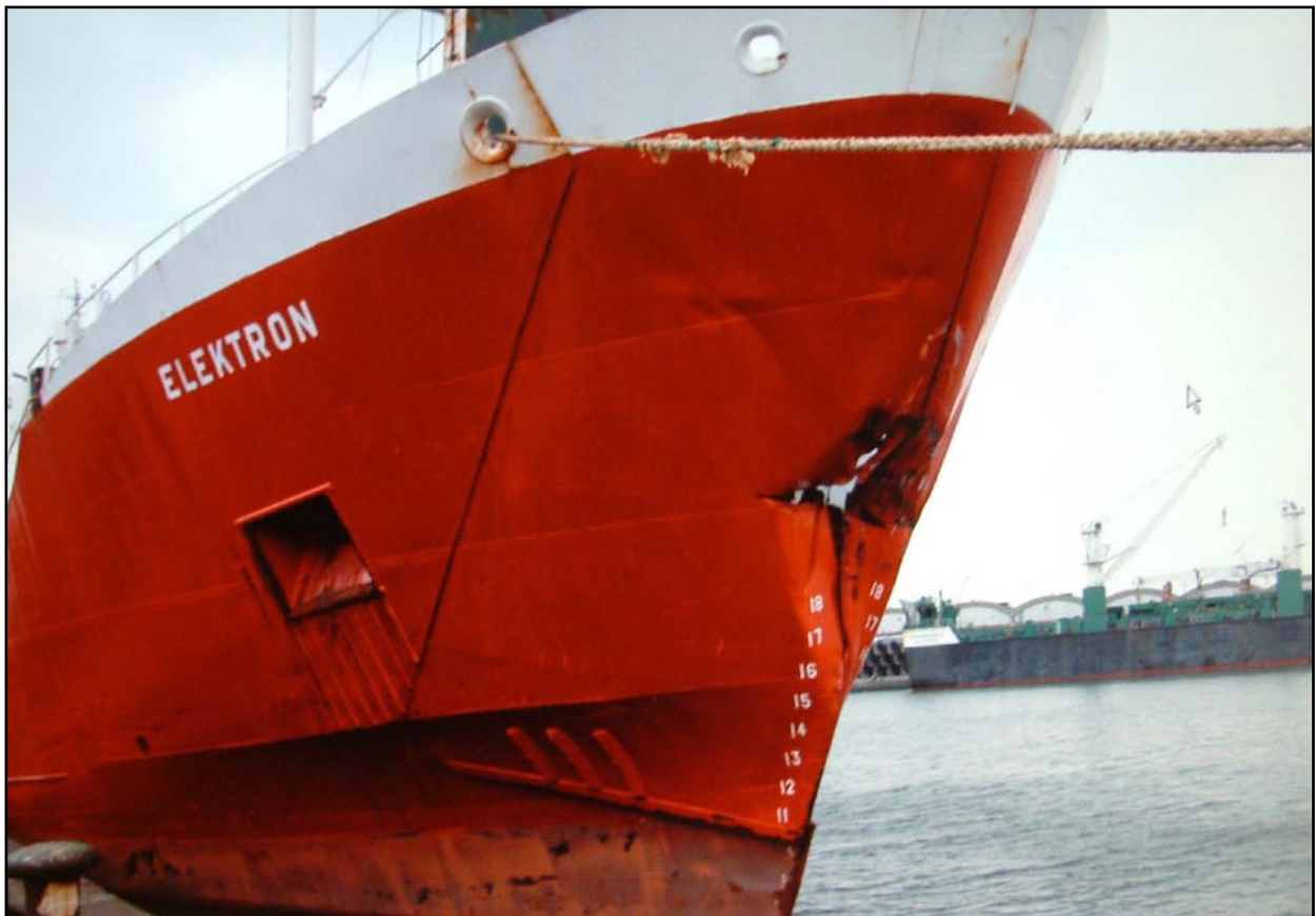
Damage to bow of Elektron , due to contact with lock gates.
