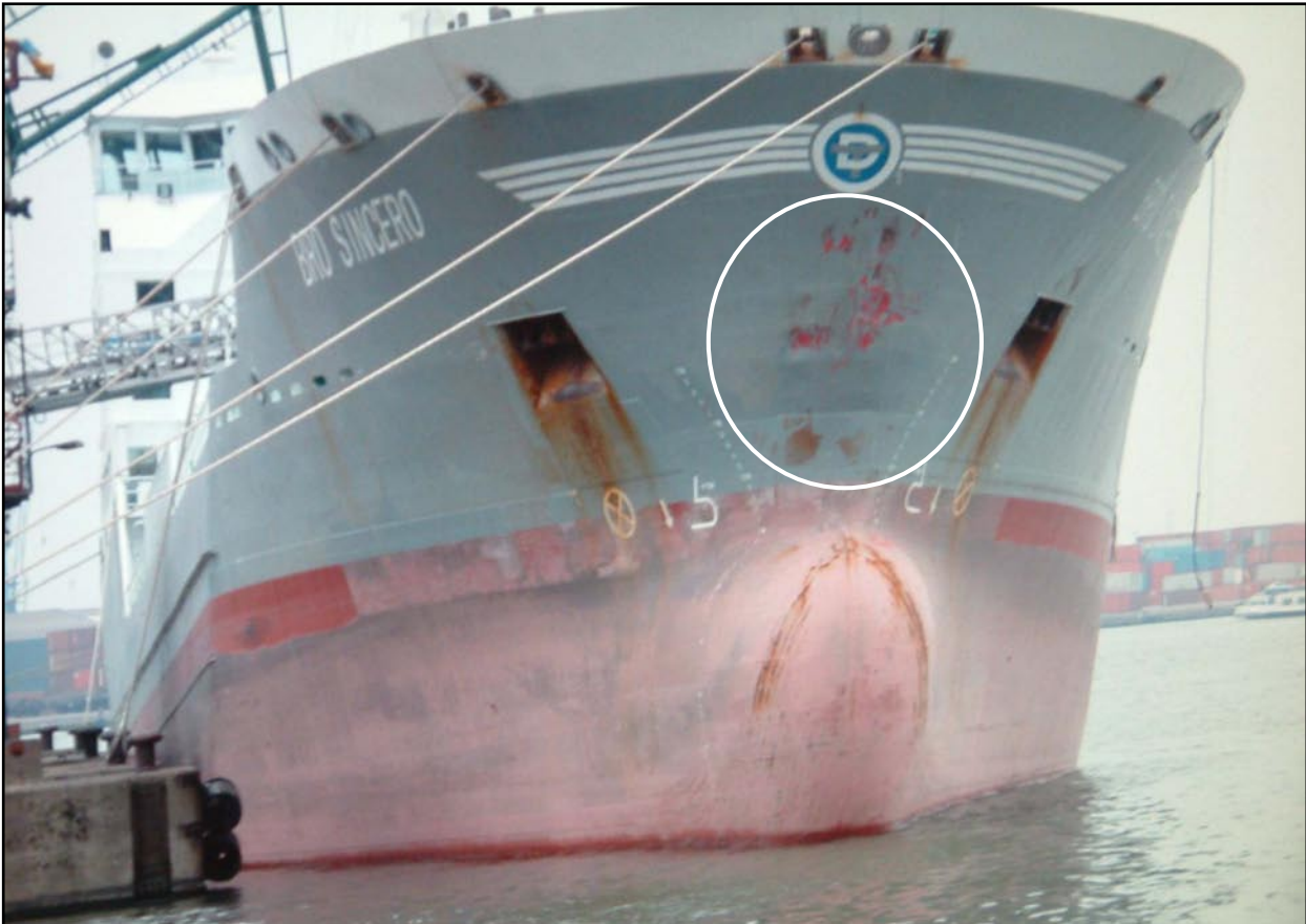
Damage to bow of Bro Sincero , due to collision with stern of Elektron .
