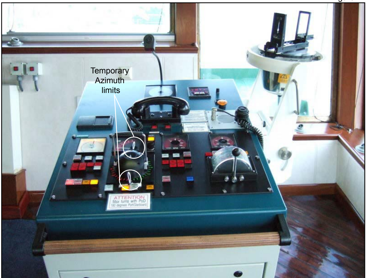
Wheelhouse starboard side console
