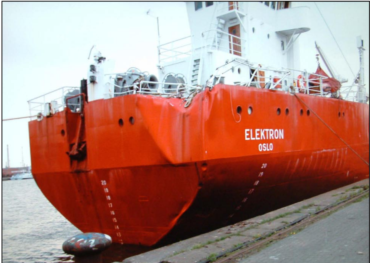
Damage to stern of Elektron , due to collision with bow of Bro Sincero
