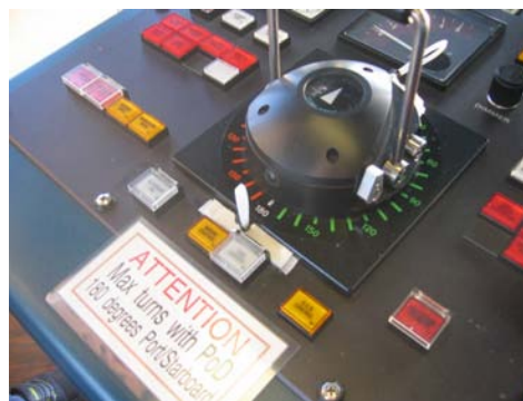
Control lever stoppers and signboard seen in stbd bridge wing, typical for all control positions.
