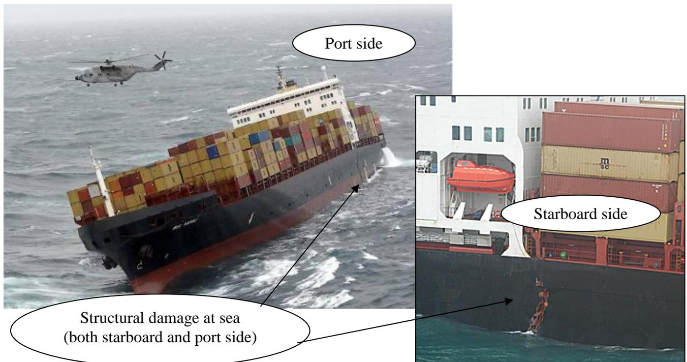
**Fig. 1.1 Structural damage in ship side. Pictures taken 18<sup>th</sup> of January 2007 after ship has been abandoned.** (with permission from Gargolaw)
