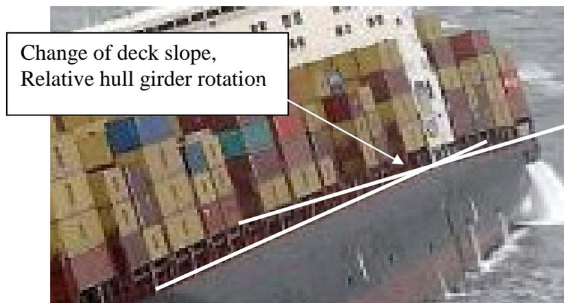
**Fig. 1.2 Structural damage in Ship side illustrating the change of deck slope at engine room bulkhead.** (with permission from Gargolaw)
