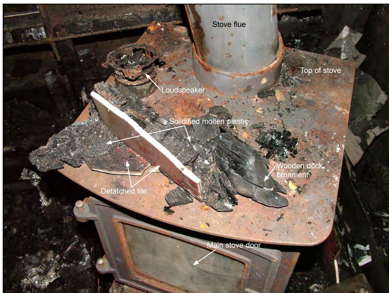
Remains of loudspeaker, wooden ornament & detached tile in situ behind the stove (14a) and recovered to the stove top (14b)
