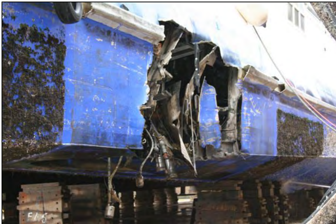
Showing damage to starboard hull of Sea express 1 once vessel dry-docked
