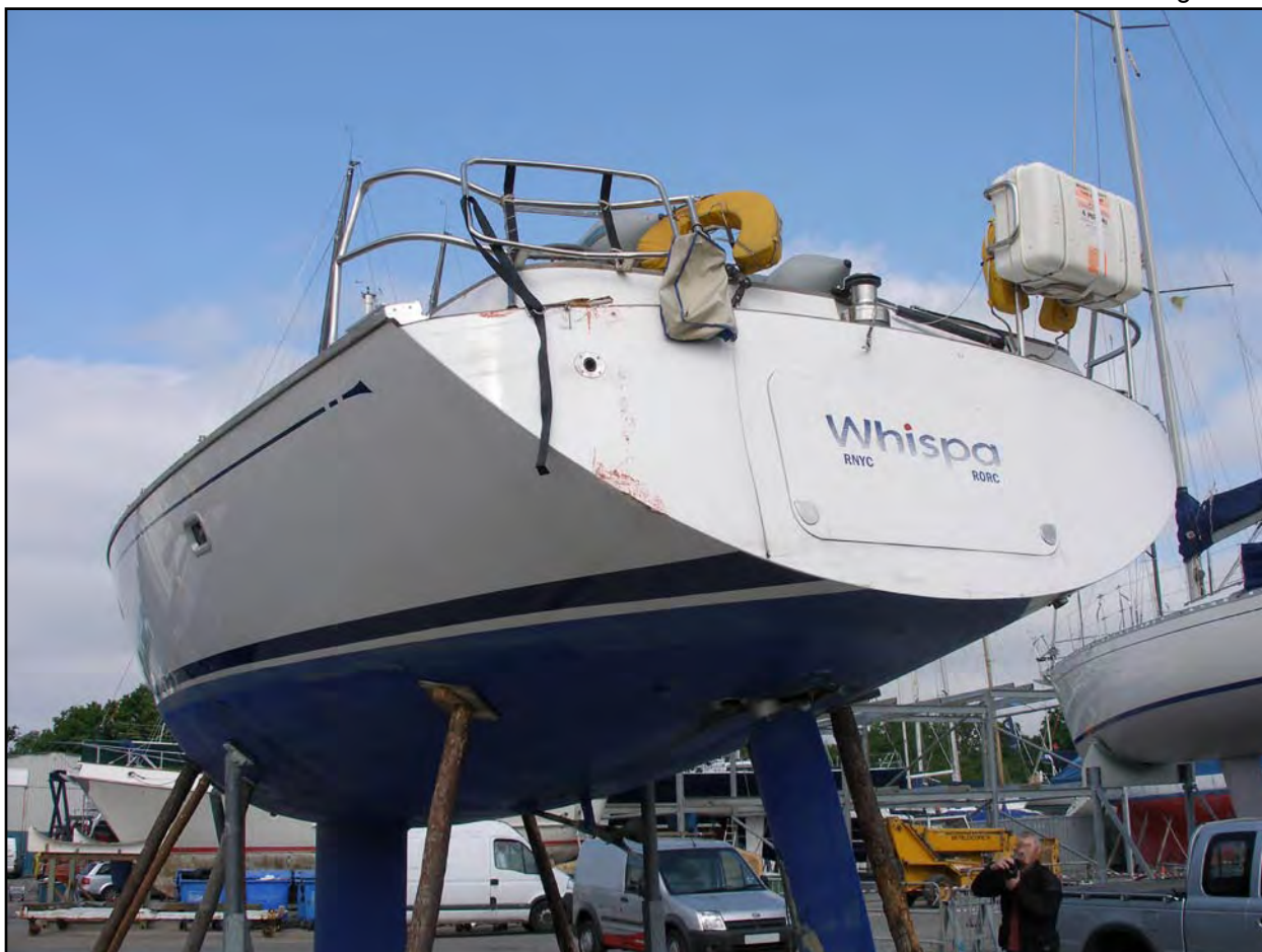
Damage to Whispa's transom and pushpit
