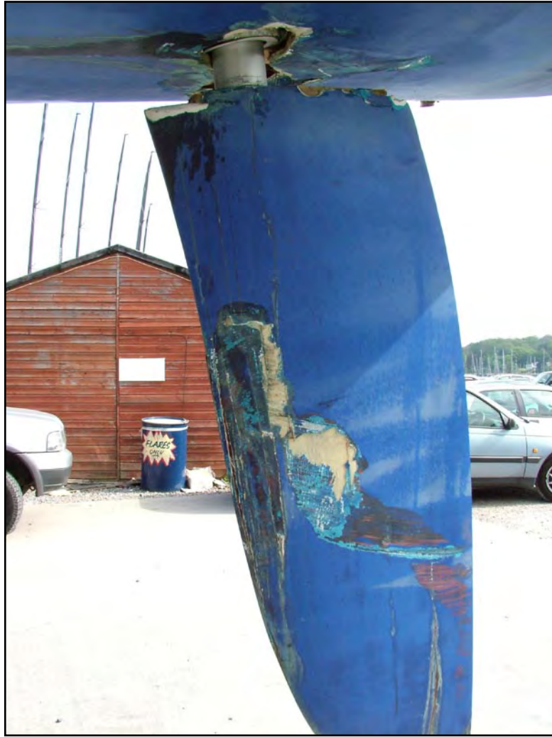
Damage to rudder by Gas Monarch's bulbous bow
