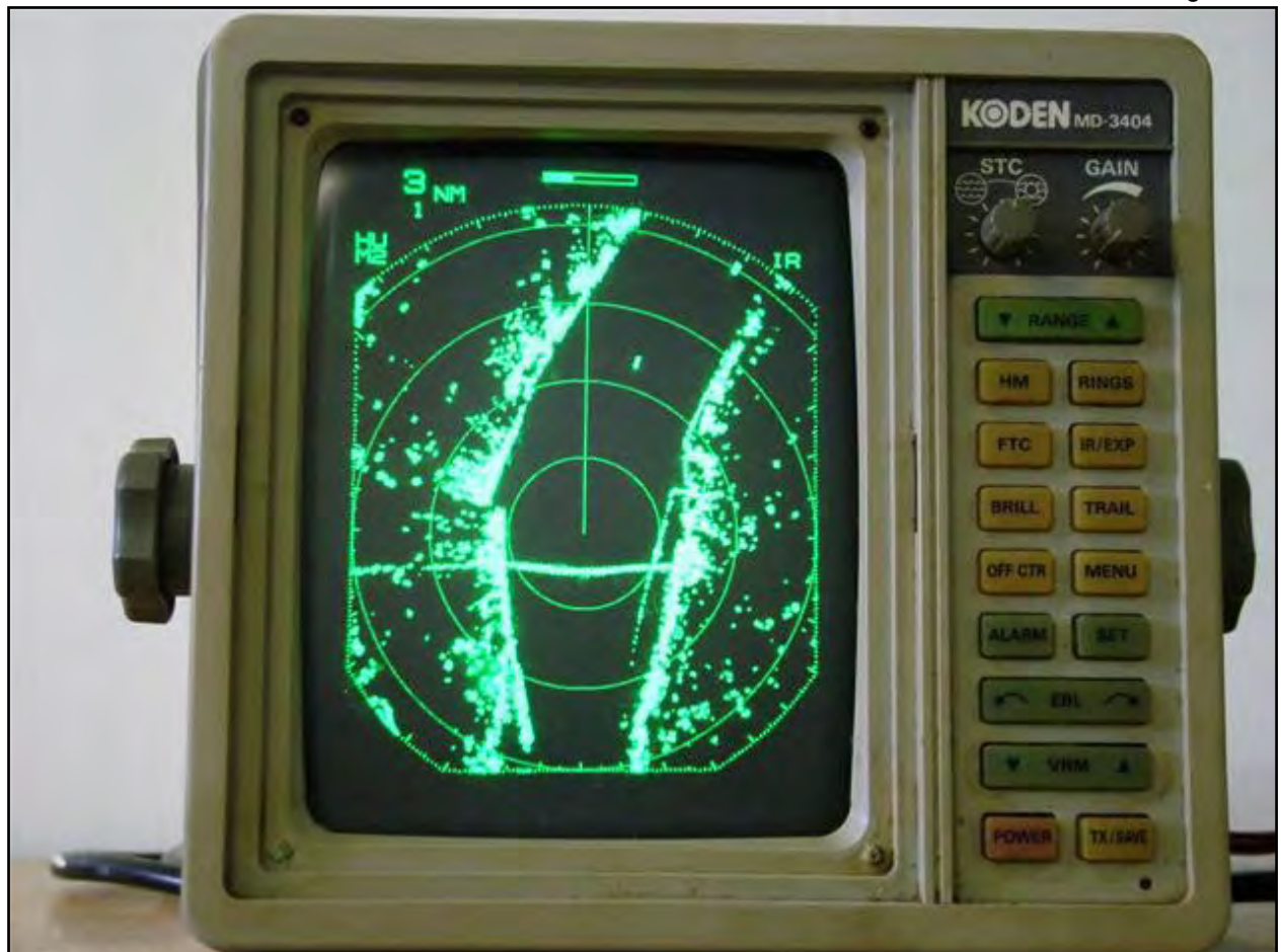
Whispa's radar screen showing 1 mile range rings on a 3 mile scale
