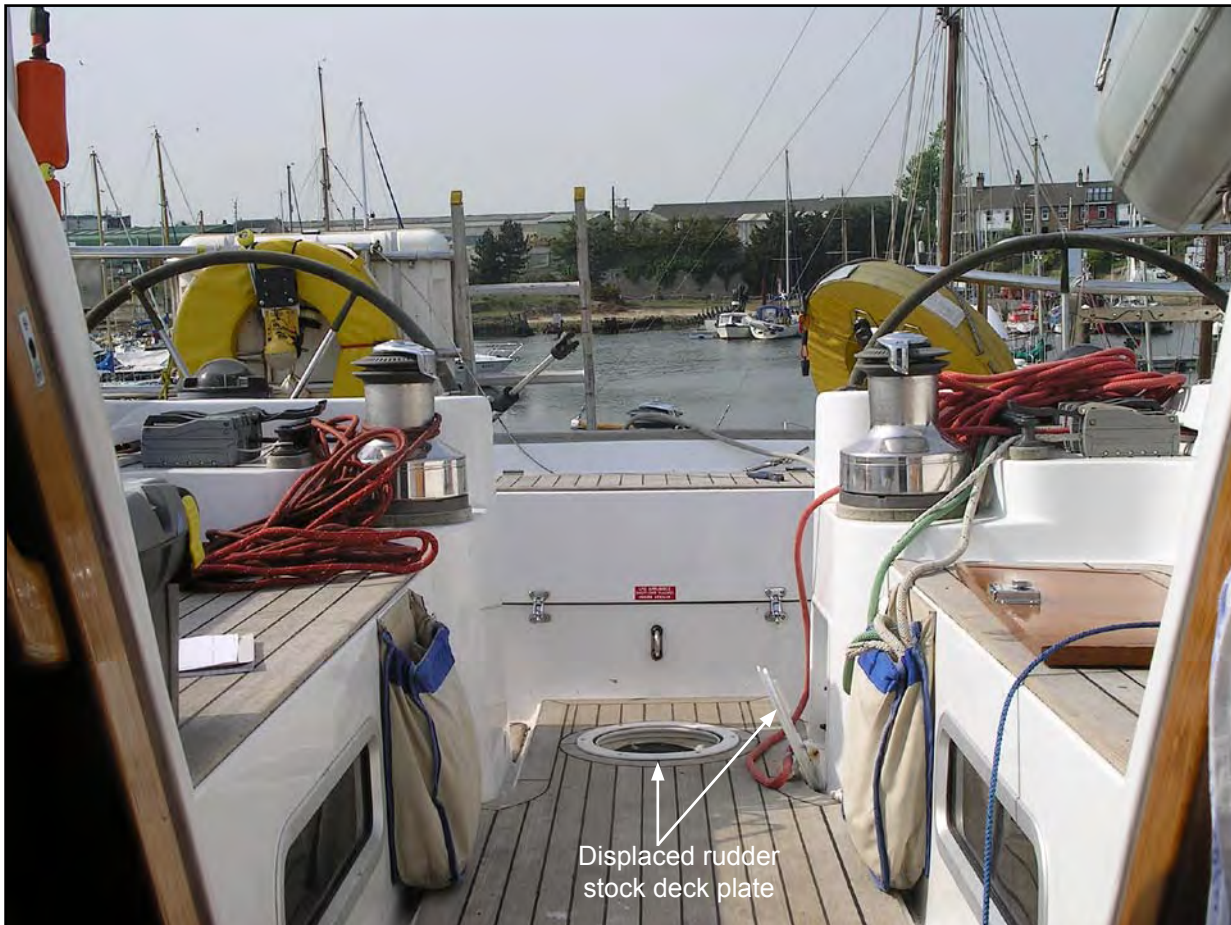
Whispa's deck, showing the displaced rudder stock deck plate
