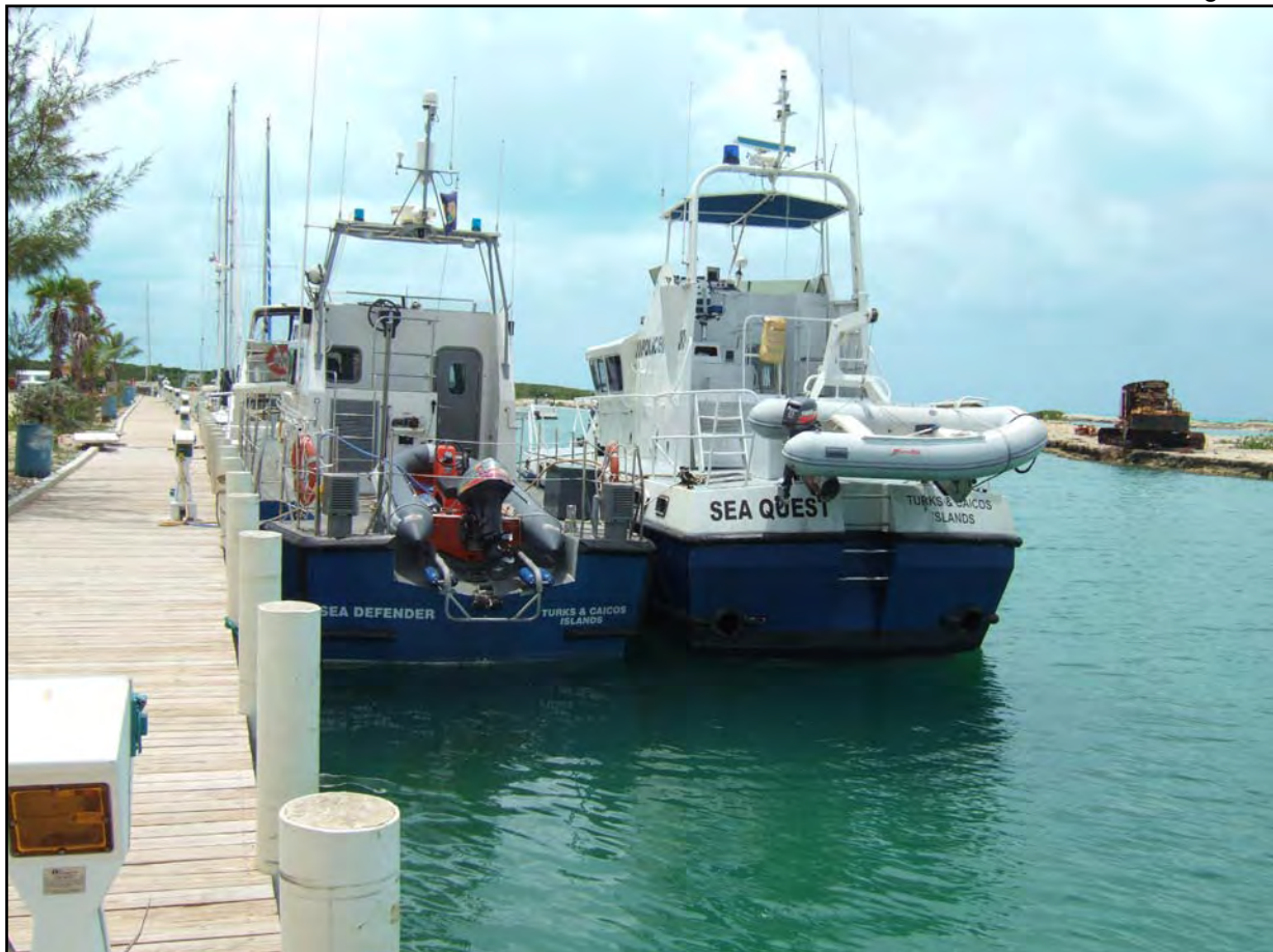
Sea Defender (left) and Sea Quest (right) showing differences in rescue craft and landing arrangements
