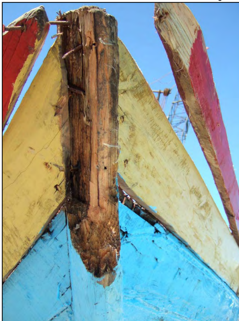
Sloop bow showing area of damage where stem head fractured
