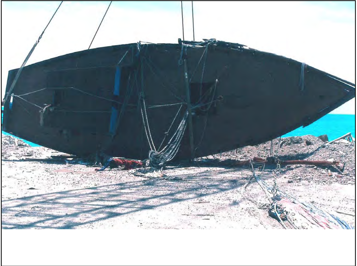
Flexing of hull as sloop lifted ashore
