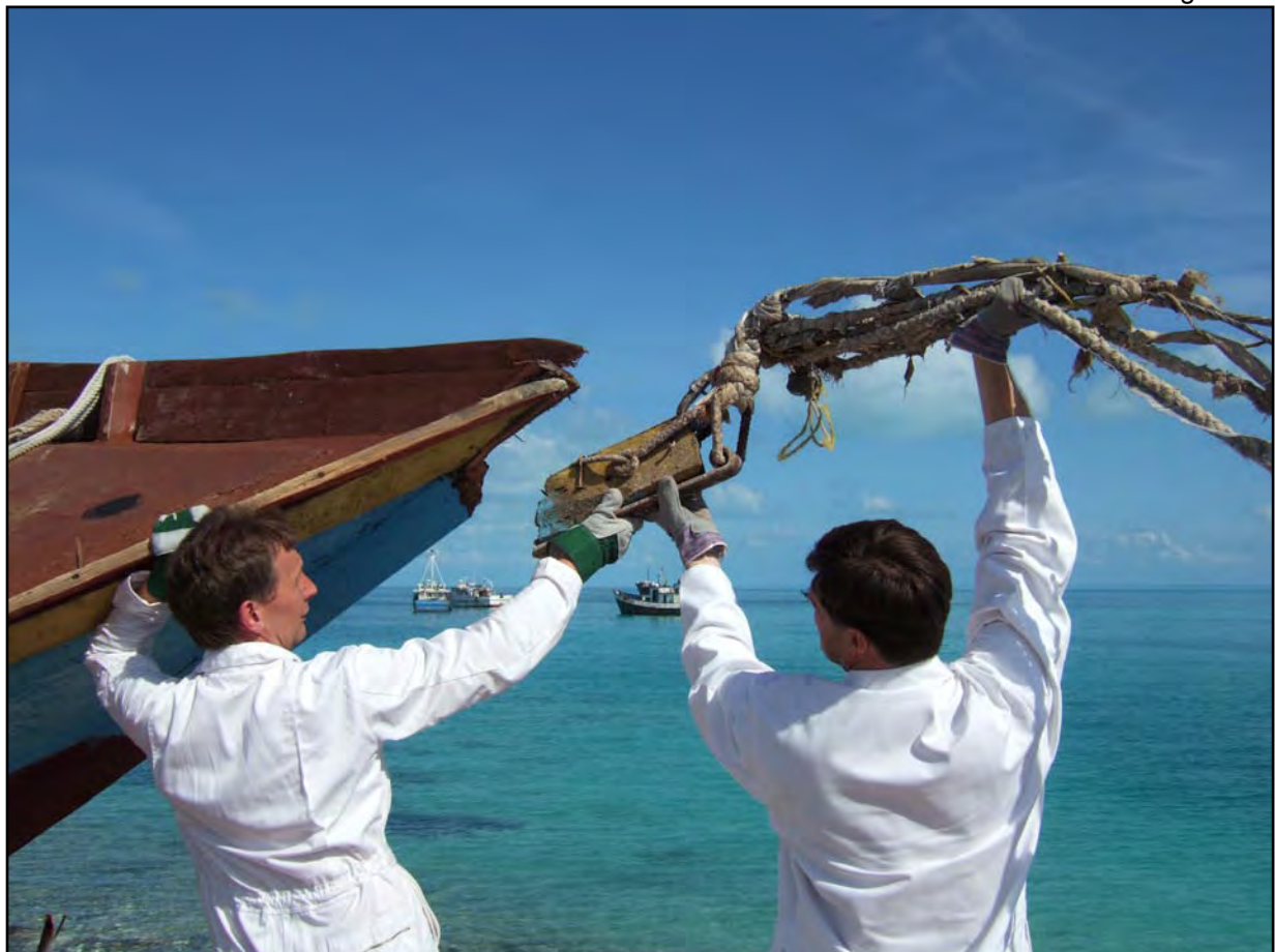
Forestays attached to broken stem head
