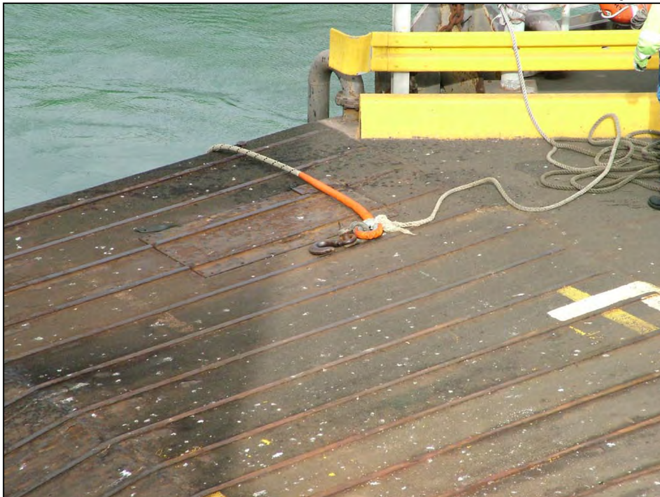
Connecting hook and messenger on shore supplied stern line
