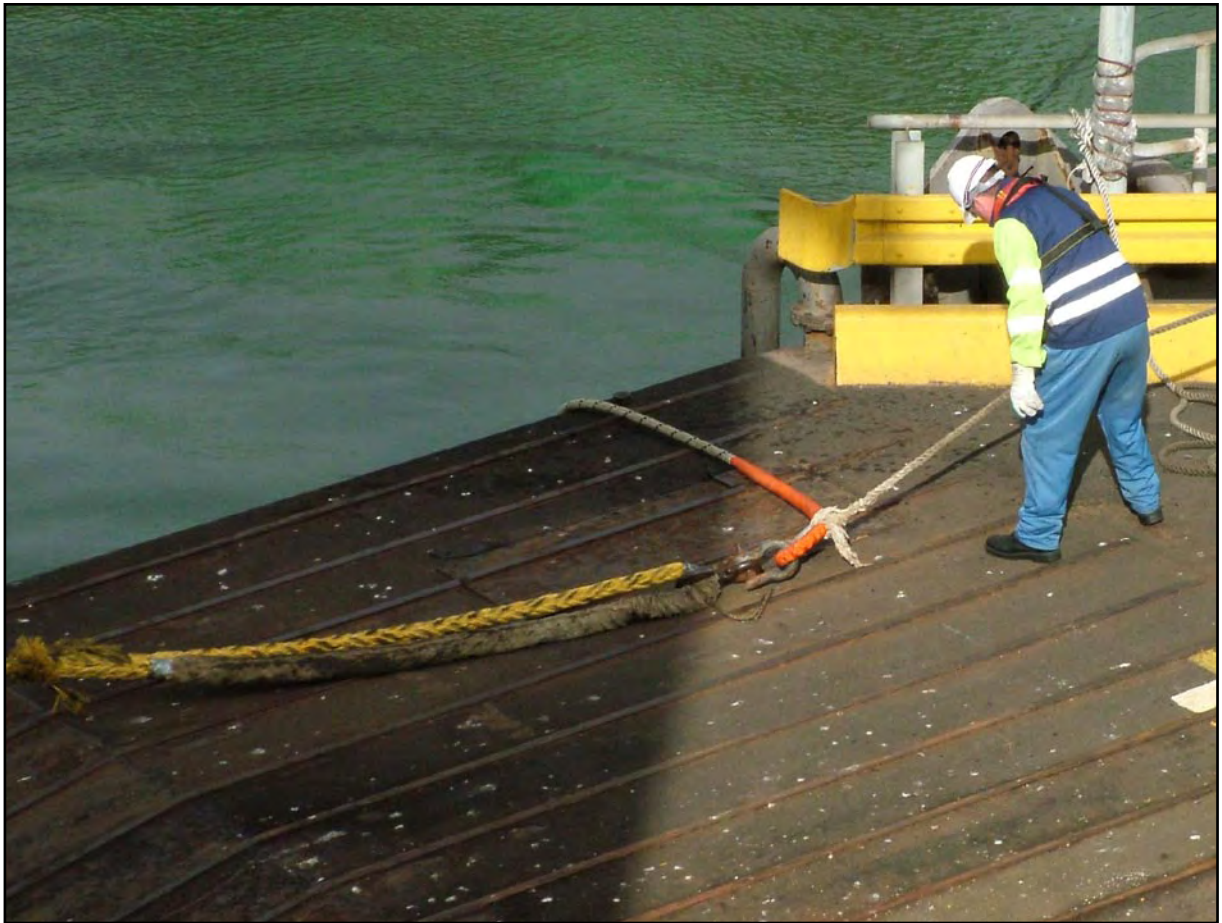
Connection between ship and shore supplied stern lines
