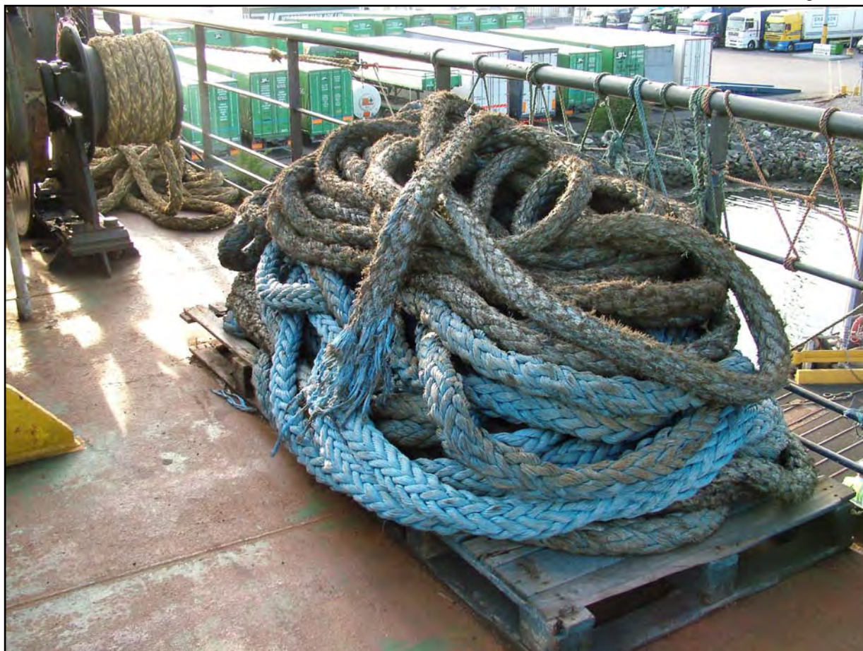
Parted stern line in normal storage position
