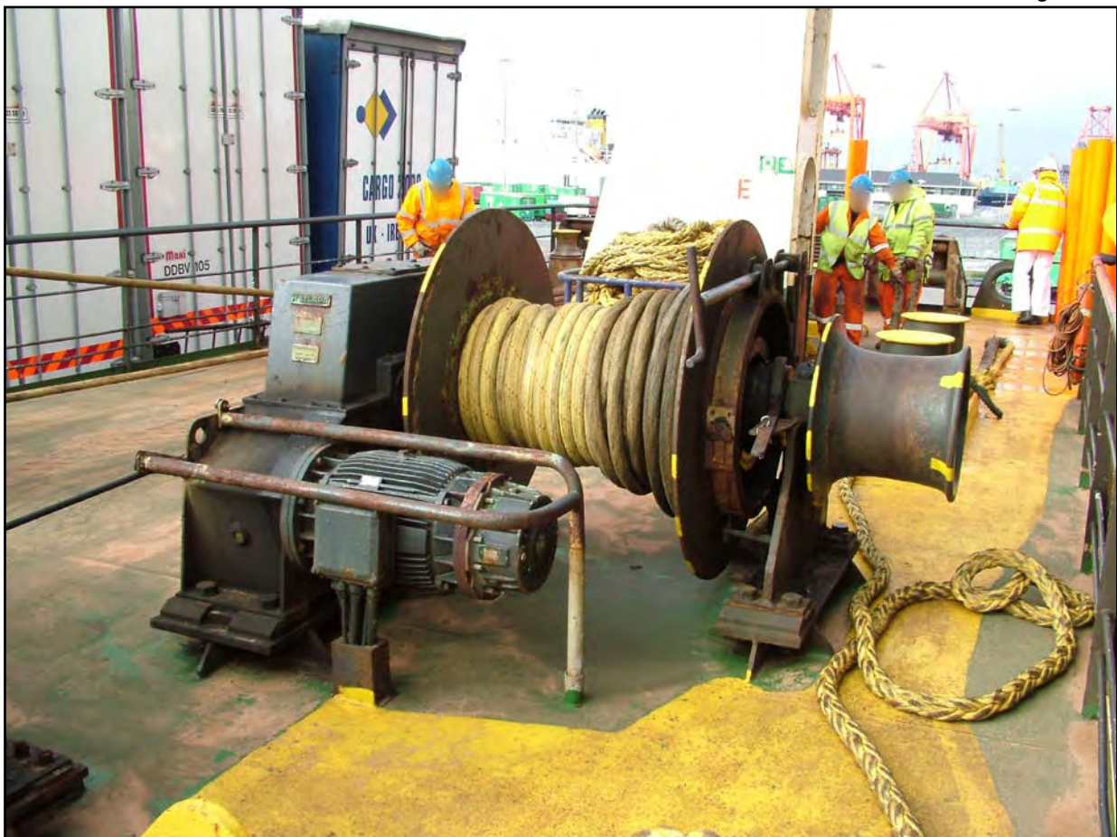
Orientation of band brake on mooring winch
