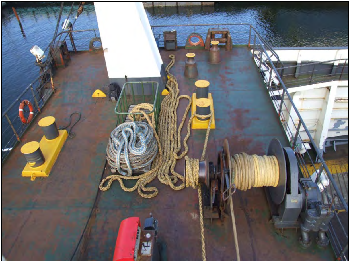
Example of methods used to secure mooring lines
