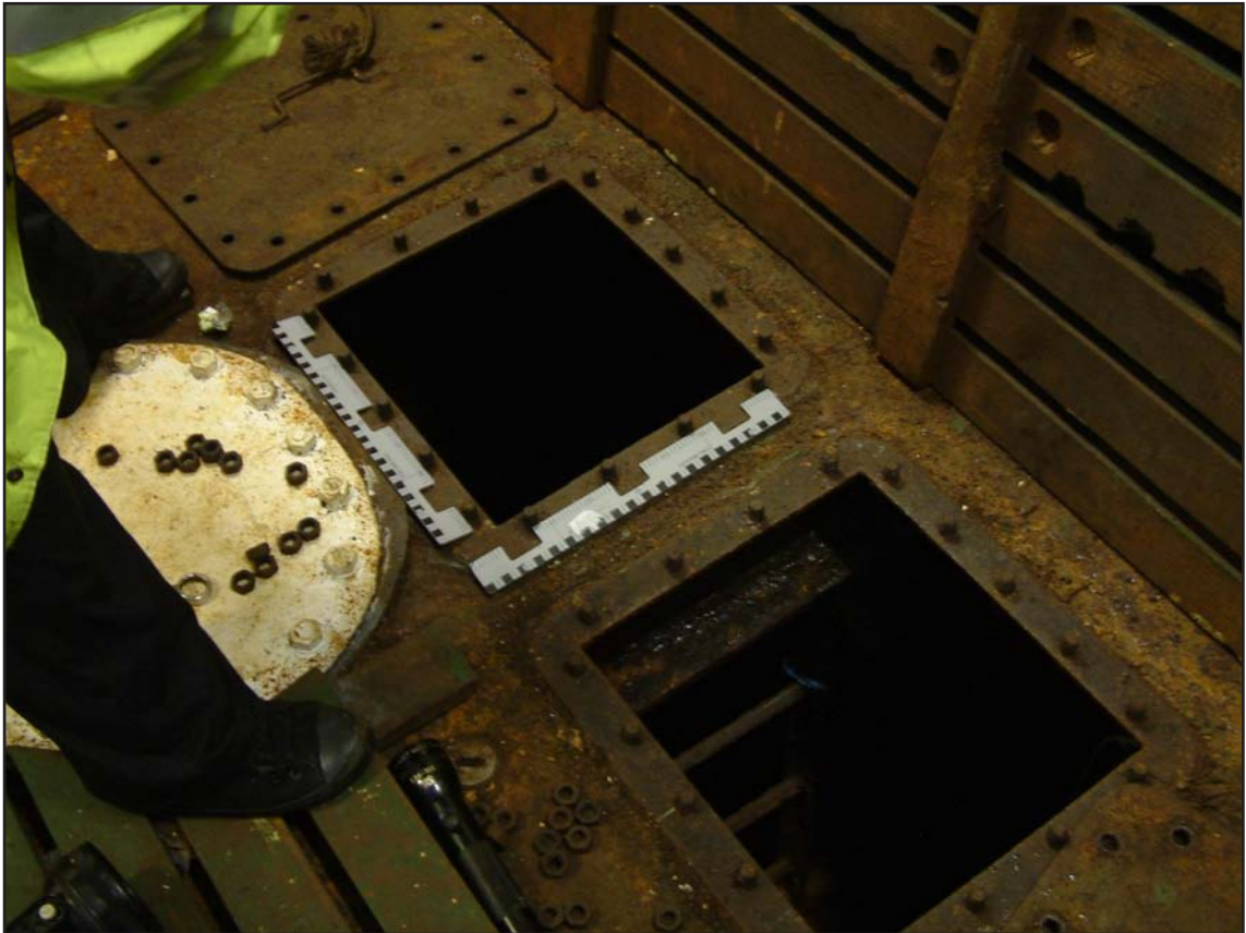
Foc'sle store - showing access hatches to chainlocker
