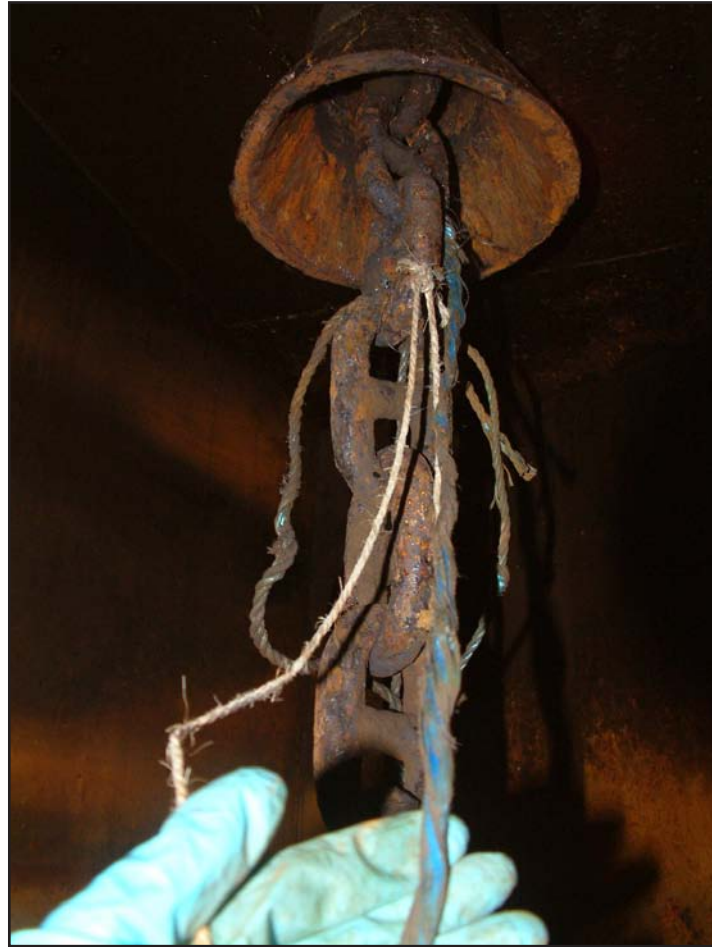
Chain locker - showing rope lashings used to stop anchor chain rattling
