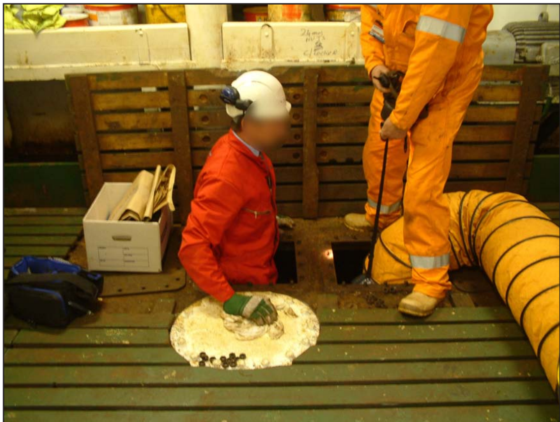
Foc'sle store - showing cramped access to chain locker
