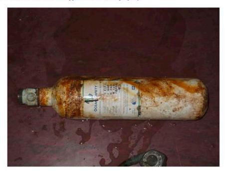
The cylinder was separately tested for leaks. Some water was removed in the cylinder before being pressurised with Carbon Dioxide.
