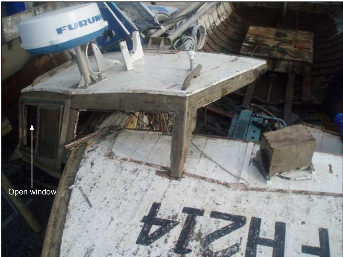
Damage to the wheelhouse of Lady Hamilton of Helford
