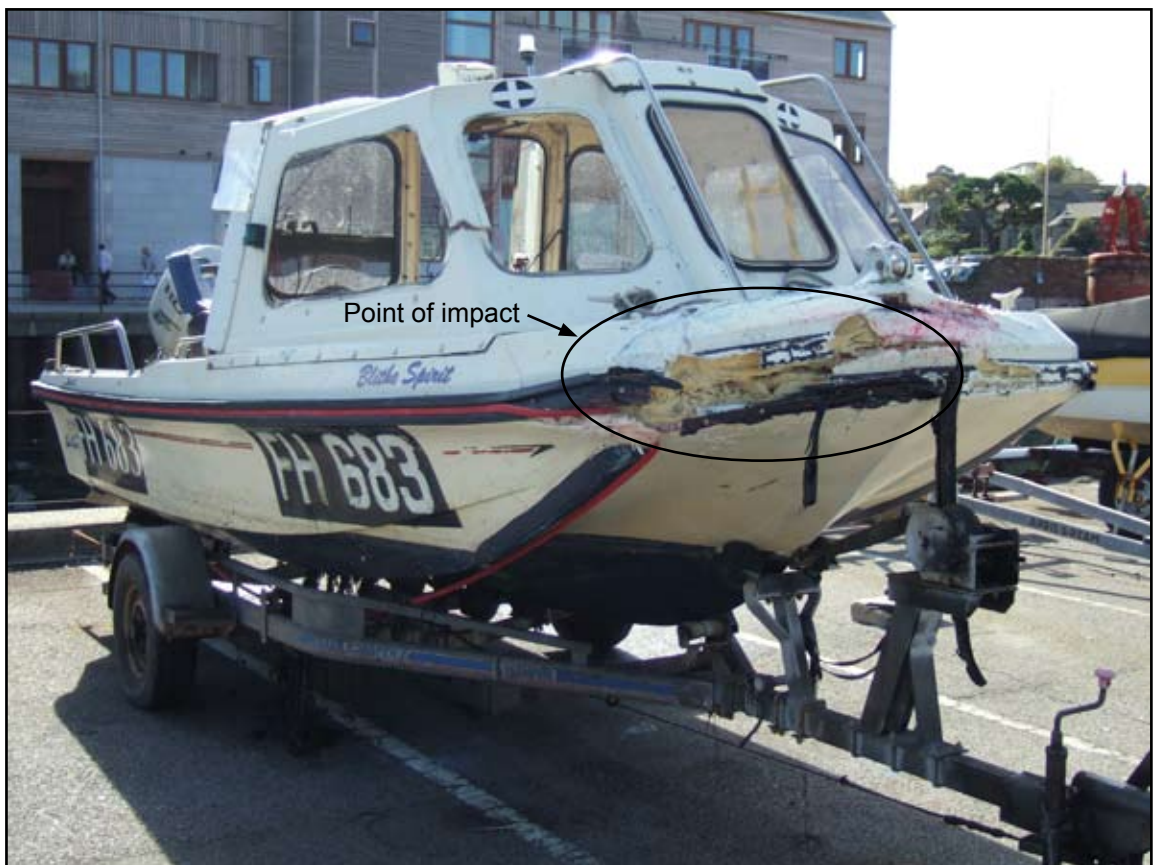
Damage to the bow of Blithe Spirit
