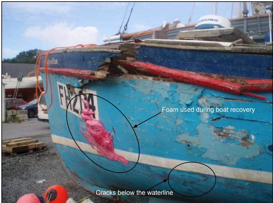
Damage to the hull of Lady Hamilton of Helford
