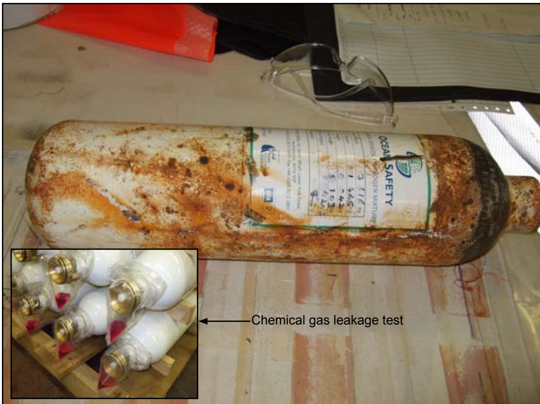
Liferaft CO 2 gas cylinder
