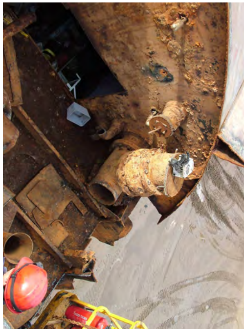
Figure 3-34 - Picture of Port heeling tank during demolition
