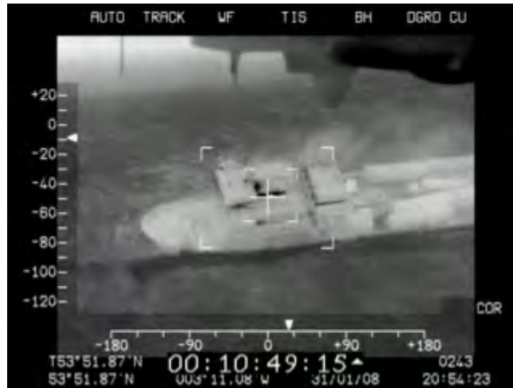
Figure 3-33 - MV RIVERDANCE at mean combined heel and list angle of 35 degrees
