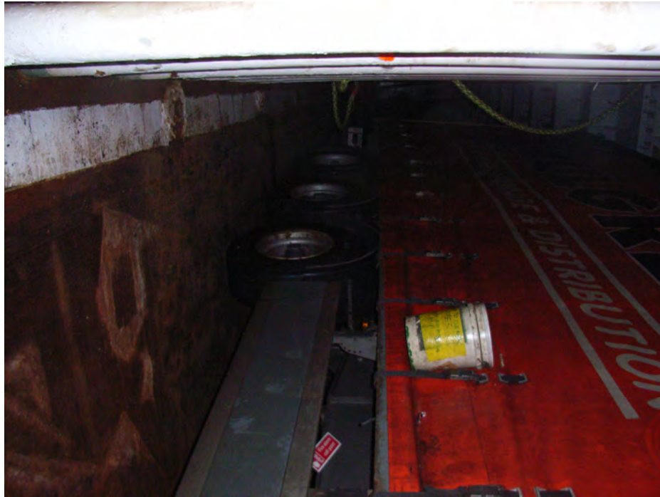
Figure 3-10 - Trailers on the Main Deck chocked against other trailers or ship's structure
