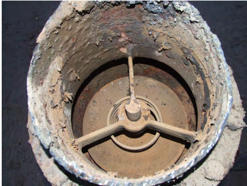
Figure 3-35 - Picture of Starboard discharge valve in the open position – note extended centre shaft
