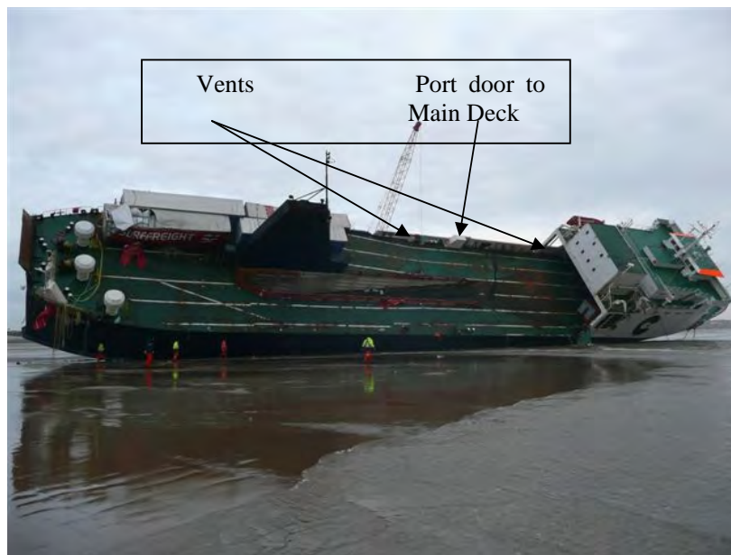
Figure 3-22 - Picture of upper (weather) deck showing potential downflooding points
