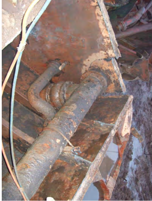
Figure 3-29 - Picture of Starboard tank suction non return valve
