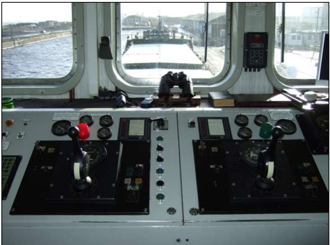
Sea Mithril's wheelhouse azimuth pod controls
