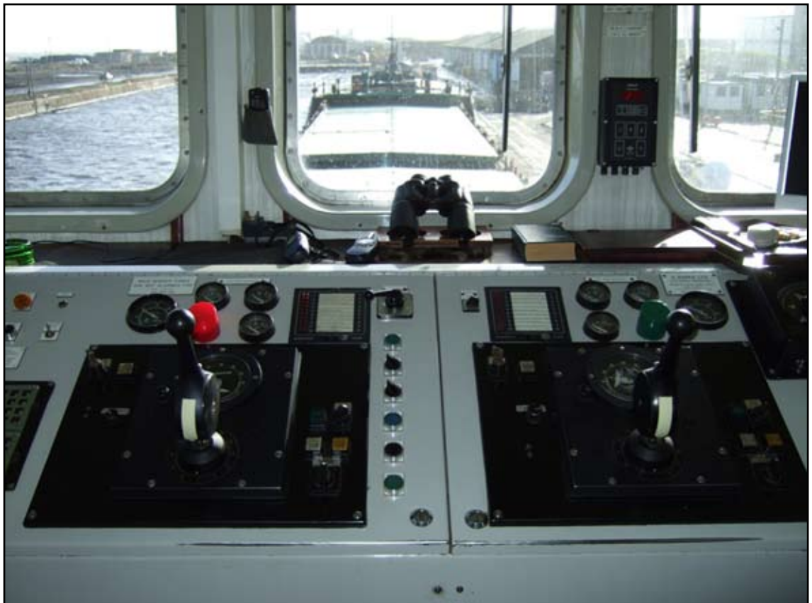
Sea Mithril's wheelhouse azimuth pod controls
