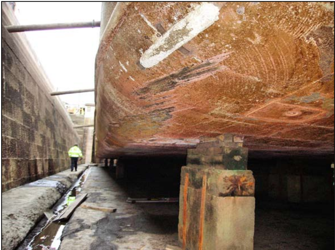
Paint damage to the underside of the hull on the vessel's port side
