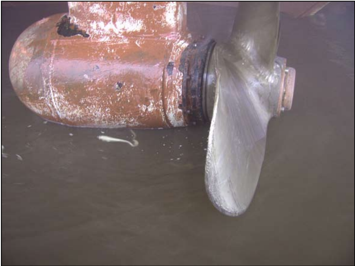
Port azimuth pod and damaged propeller
