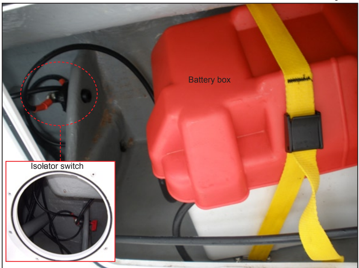
Partner 1 battery box and electrical isolator switch
