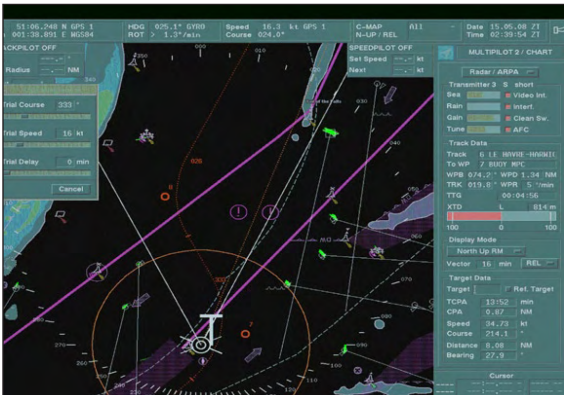
Trial manoeuvre carried out by Costa Atlantica at 0239
