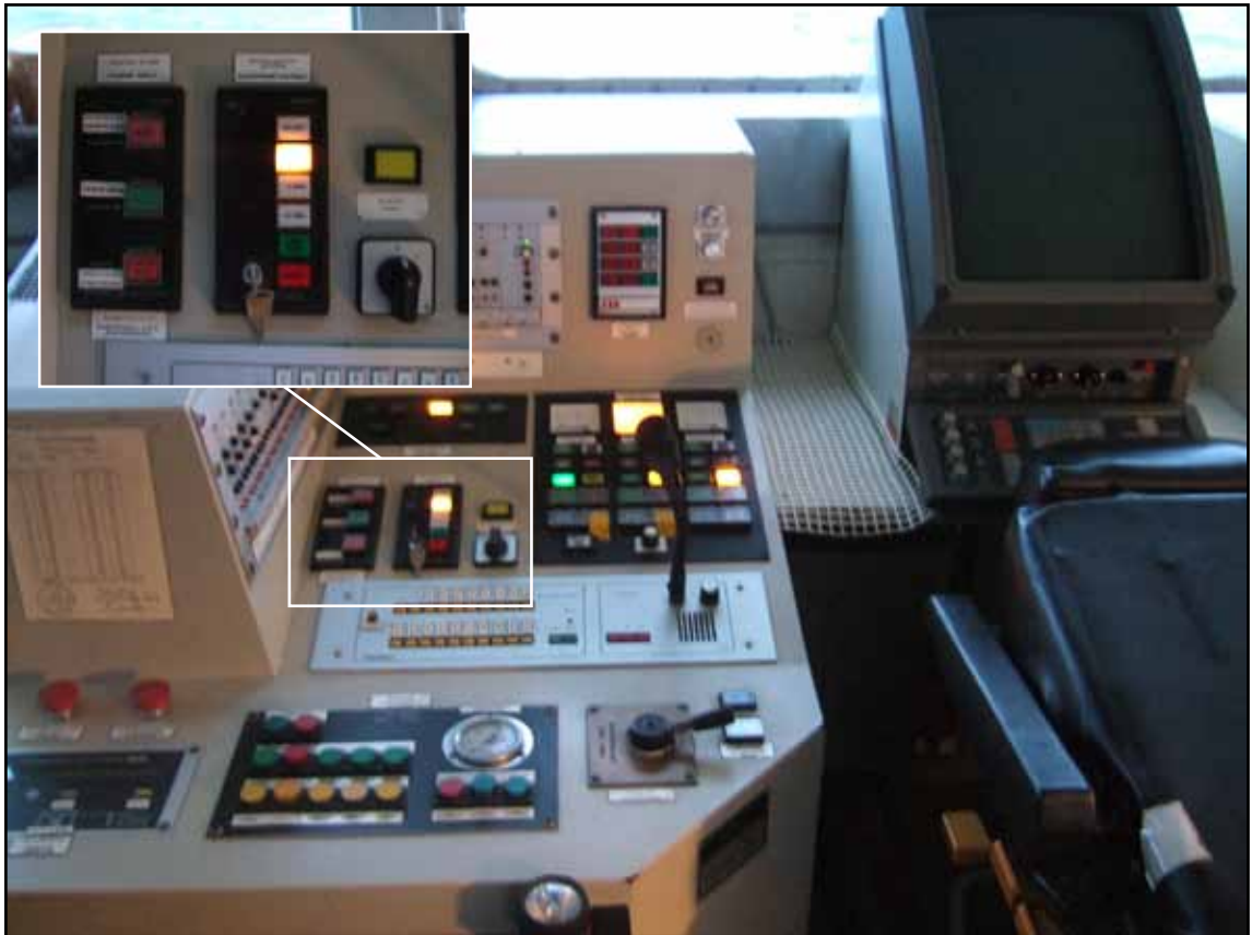
Watch alarm in wheelhouse
