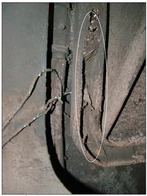
Cross alleyway, port watertight door - heat damaged seal
