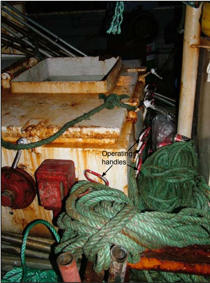
Figure 24 Quick shut-off valve operating gear obstructed by bundles of ropes
