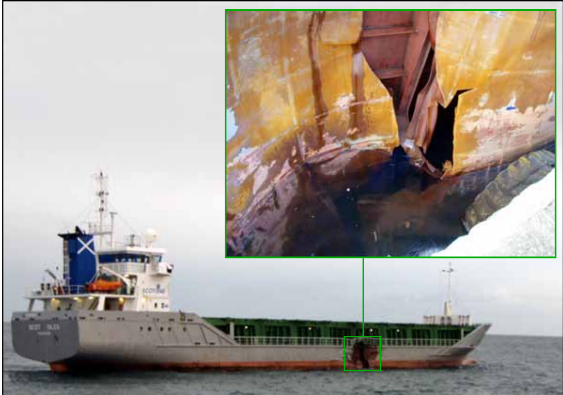
Scot Isles - damage overview
