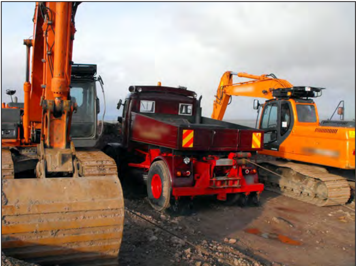
Winches and excavators used to keep Abigail H upright during the salvage operations
