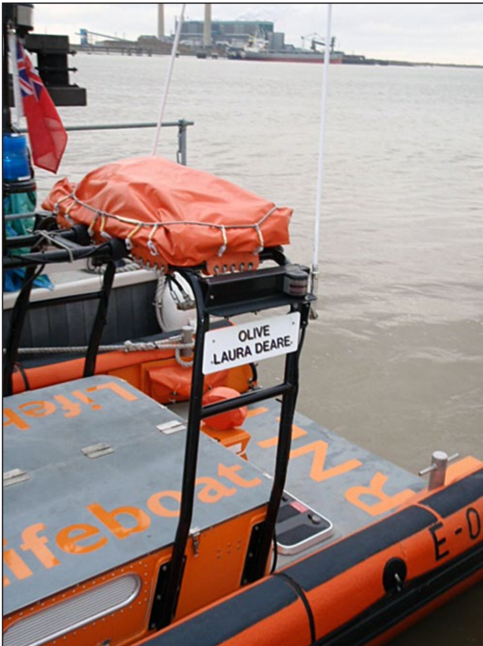
Low transom of RNLI lifeboat used to recover the casualty from the water
