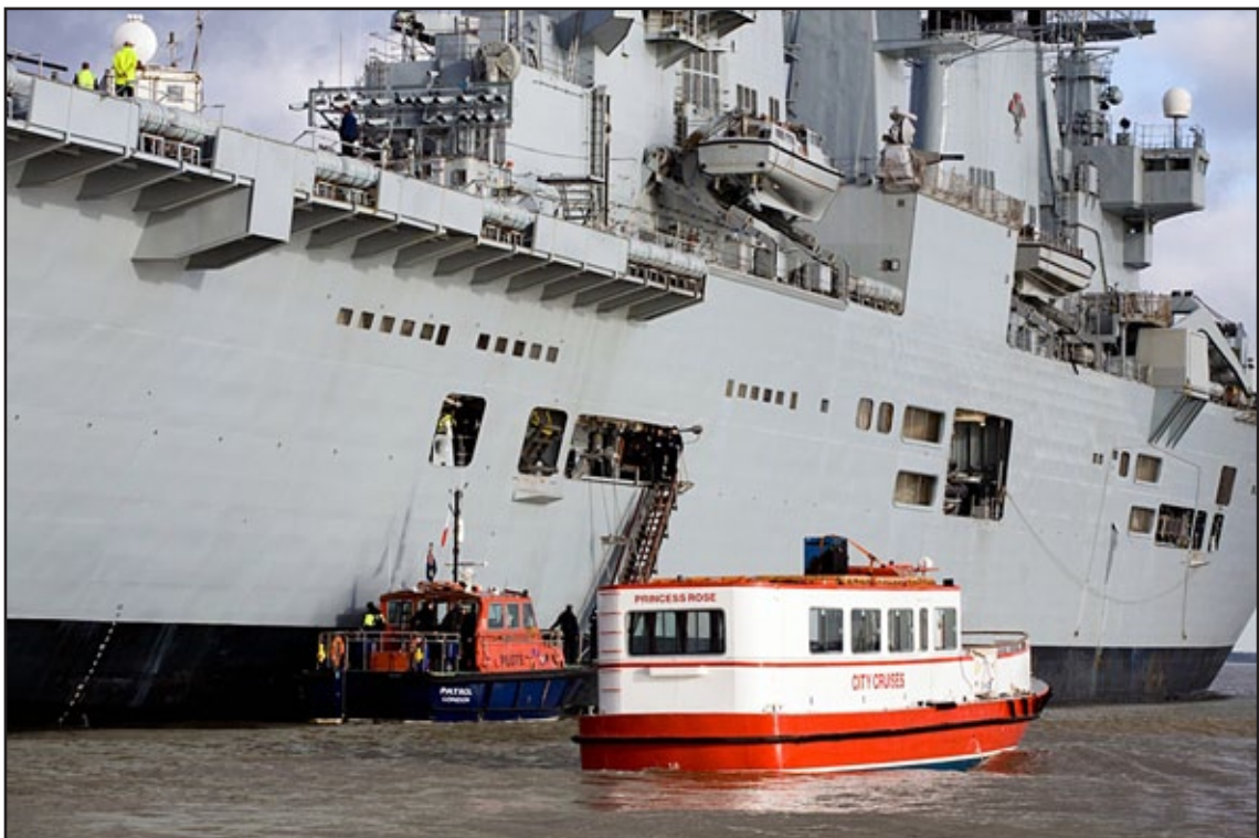
Example of an underway passenger transfer at slow speed using an accommodation ladder
