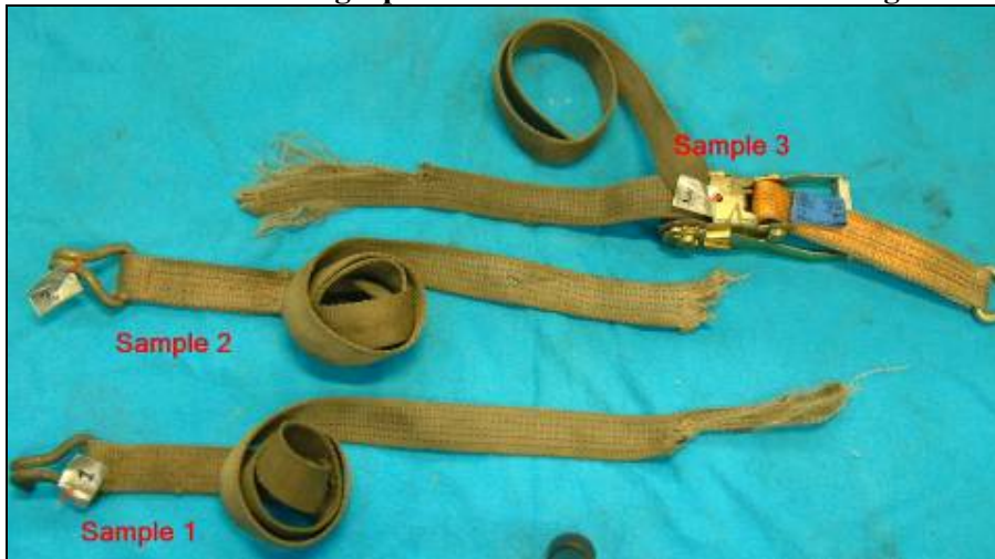
Photograph 1 General view of failed lashings
