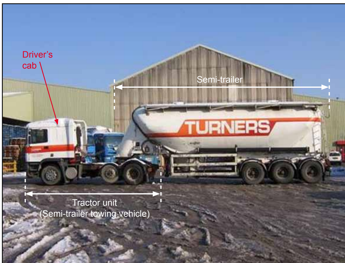
Turners (Soham) Ltd bulk powder articulated road tanker
