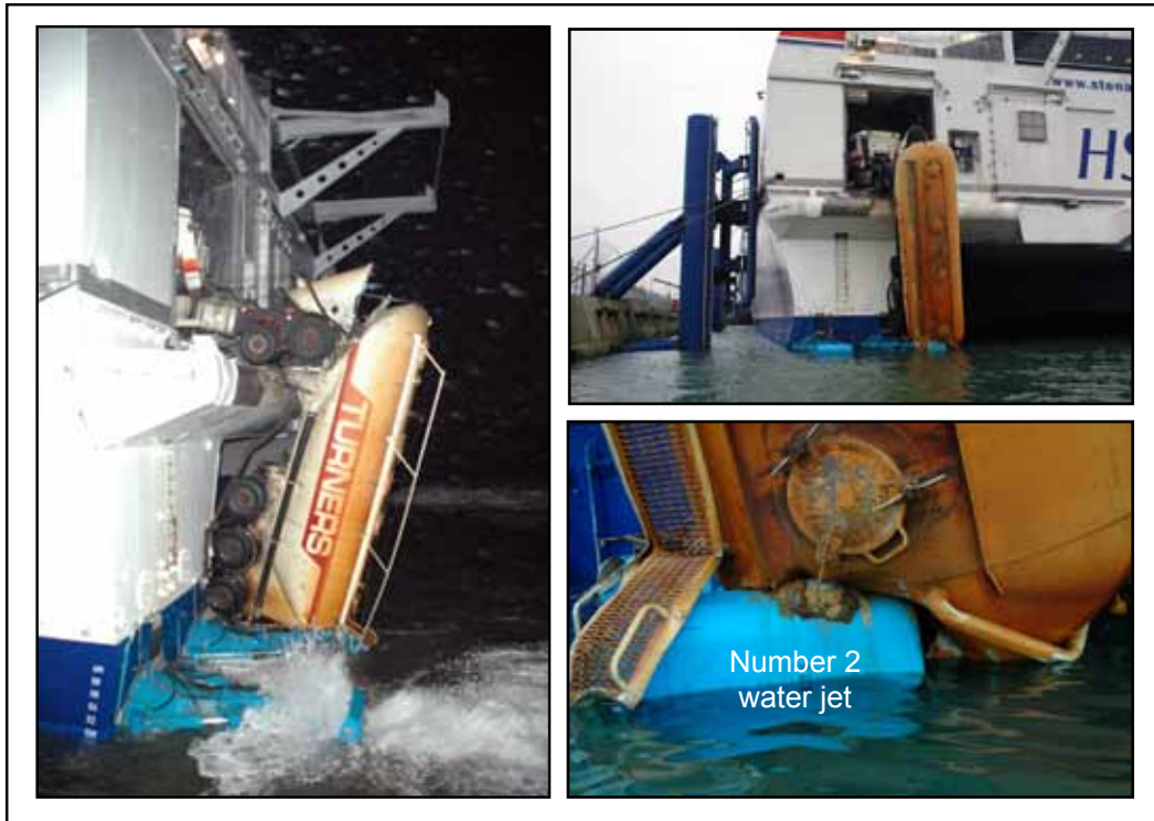
Road tanker semi-trailer resting on top of number two water jet
