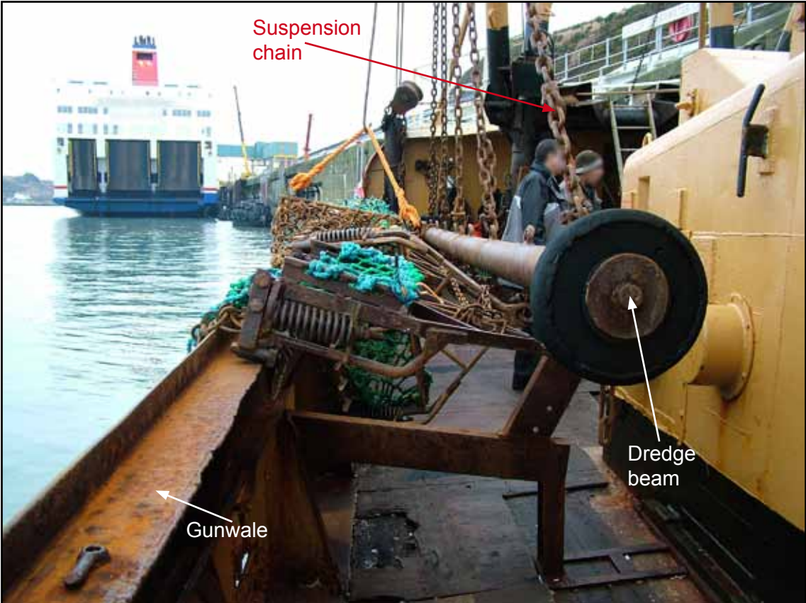
Simulated position of dredge beam at time of accident
