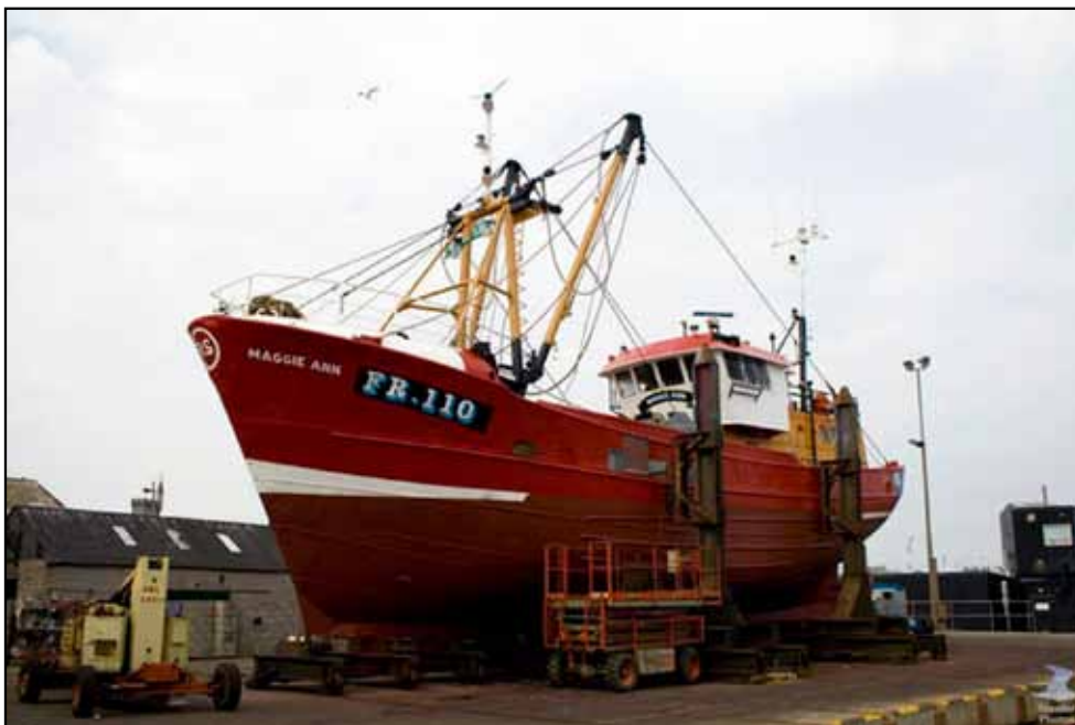
Maggie Ann - showing modification to the bulwark
