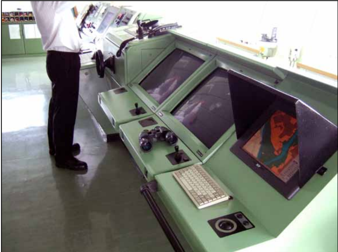
Pilot's position next to the starboard radar display
