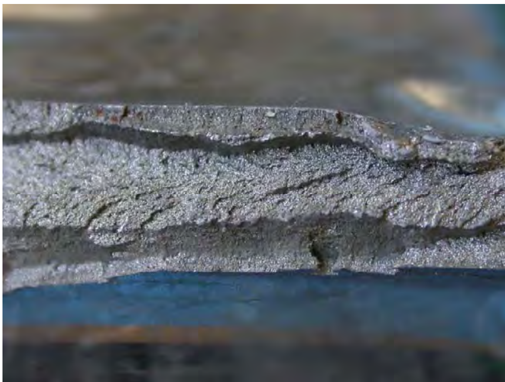
Figure 27: Sixth region of the cylinder block fracture surface, showing features consistent with a single event brittle fracture (post fracture mechanical damage noted).
