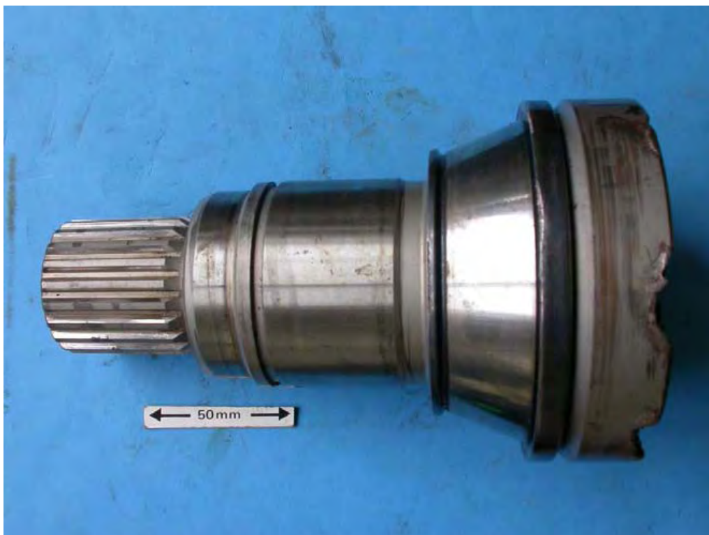
Figure 49: Motor output shaft, which was supplied retaining the inner raceway cone from one of the shafts two rolling element bearings.
