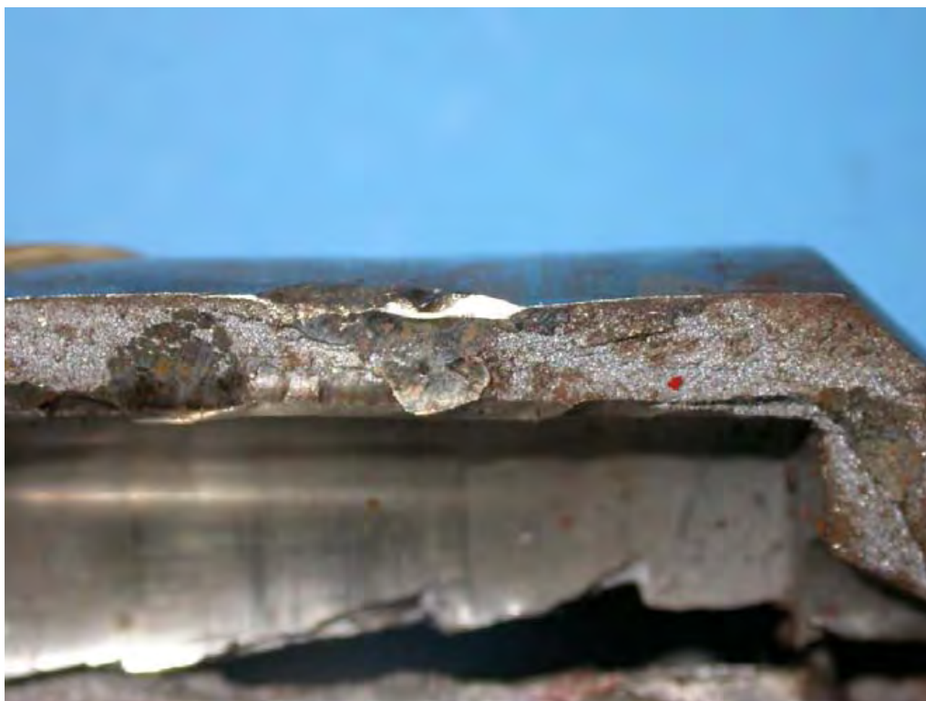
Figure 11: Typical sites of post fracture impact damage.
