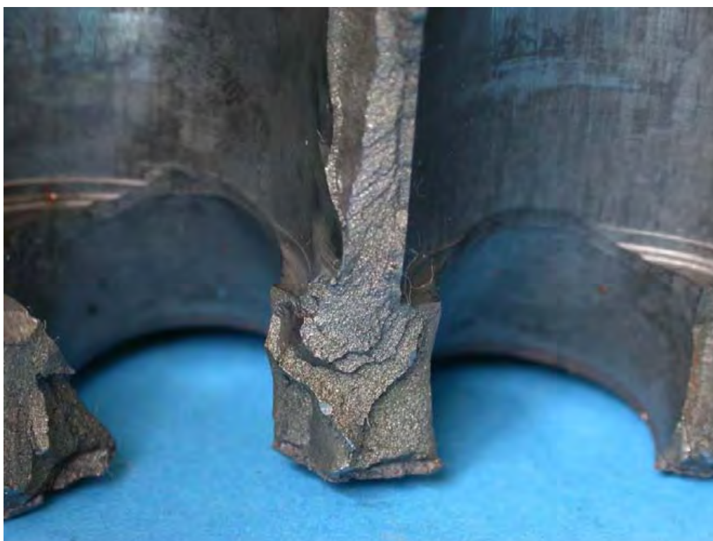
Figure 22: Region of the cylinder block fracture surface, showing features consistent with a single event brittle fracture (post fracture mechanical damage noted).
