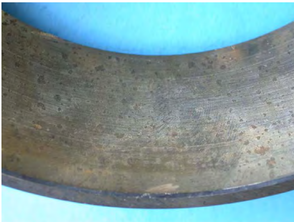
Figure 53: Outer raceway ring from the larger of the two shaft bearings, which exhibited no evidence of severe wear or damage.
