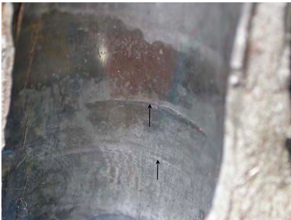
Figure 19: Detail of piston mechanical indenting damage (arrowed) at the walls of a second cylinder.
