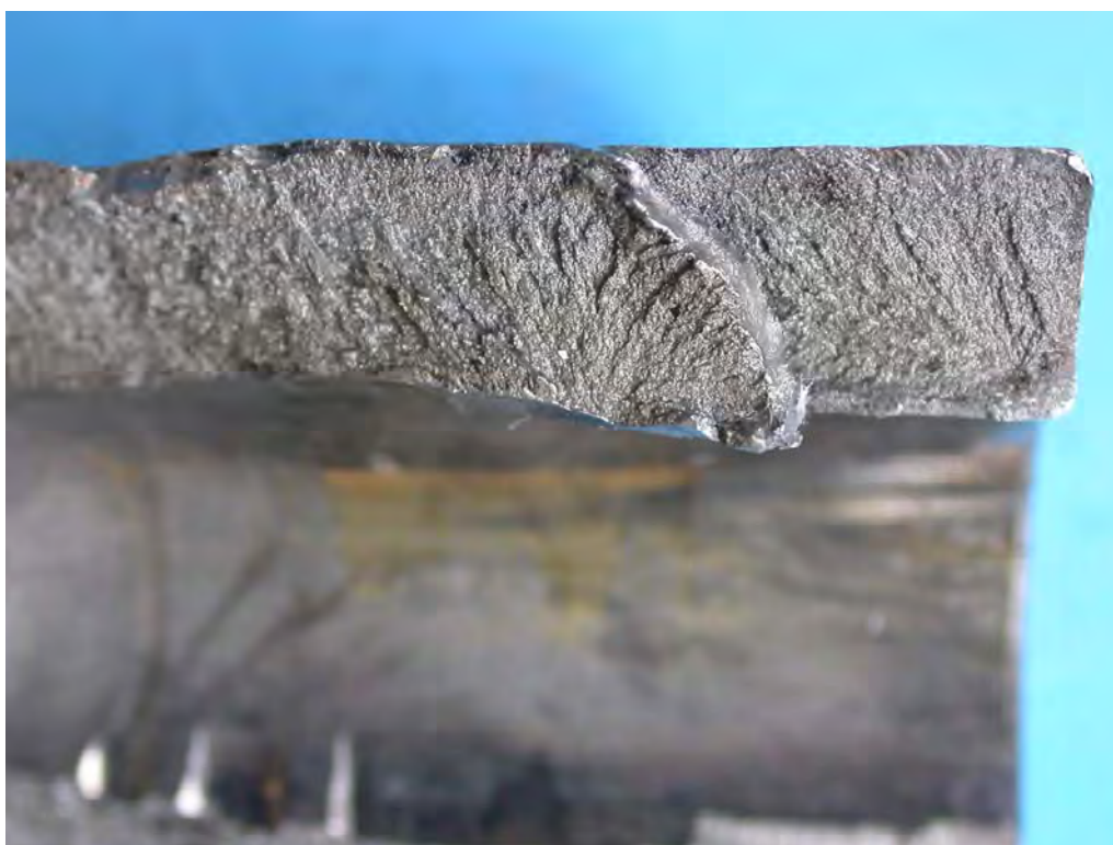
Figure 26: Fifth region of the cylinder block fracture surface, showing features consistent with a single event brittle fracture (post fracture mechanical damage noted).
