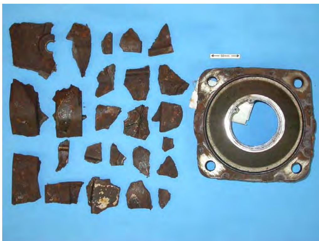
Figure 56: Recovered pieces from the extensively fractured cast iron motor casing.
