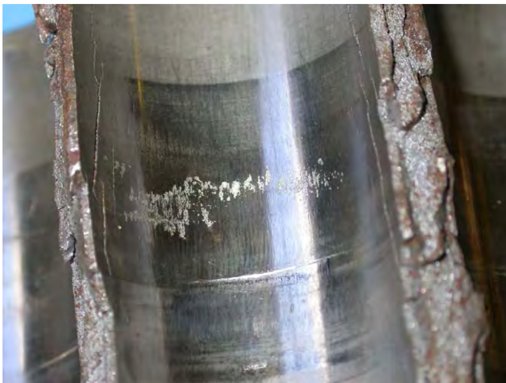
Figure 21: Incipient cylinder bore wear or spalling type damage.
