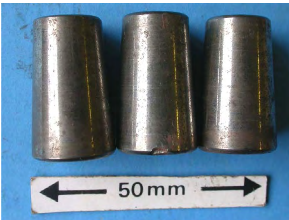
Figure 52: Three rollers recovered from the larger of the two shaft bearings, which exhibited no evidence of wear or pre-casualty damage.
