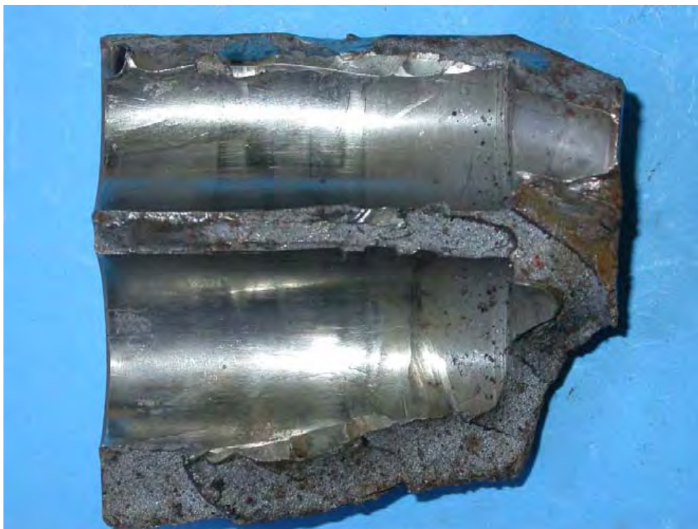
Figure 9: Third of the recovered cylinder block pieces, showing the orientation and locations of the fracture sites (post fracture impact damage noted).
