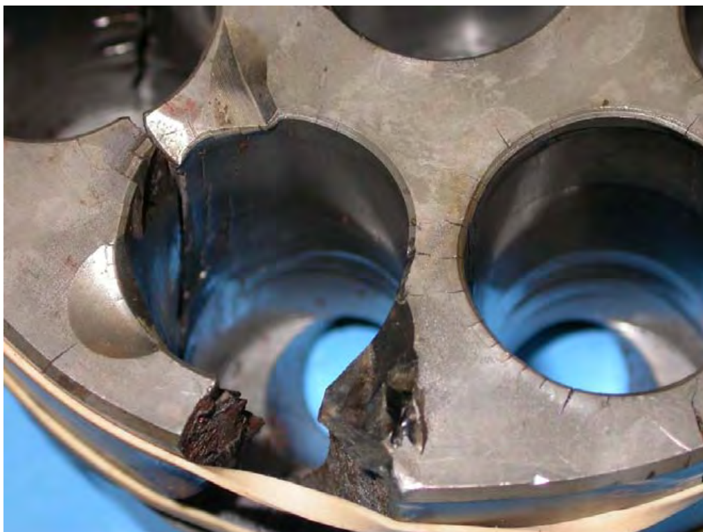
Figure 15: Detail of output end secondary radial cracks at two further adjacent cylinder sites
