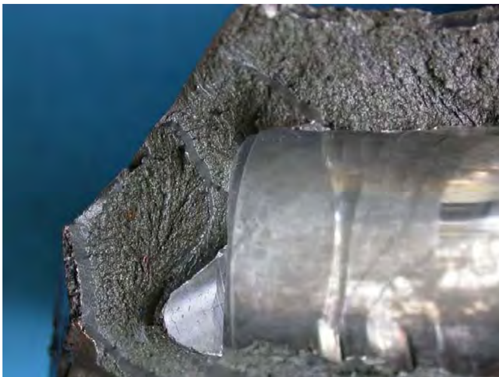
Figure 23: Second region of the cylinder block fracture surface, showing features consistent with a single event brittle fracture (post fracture mechanical damage noted).
