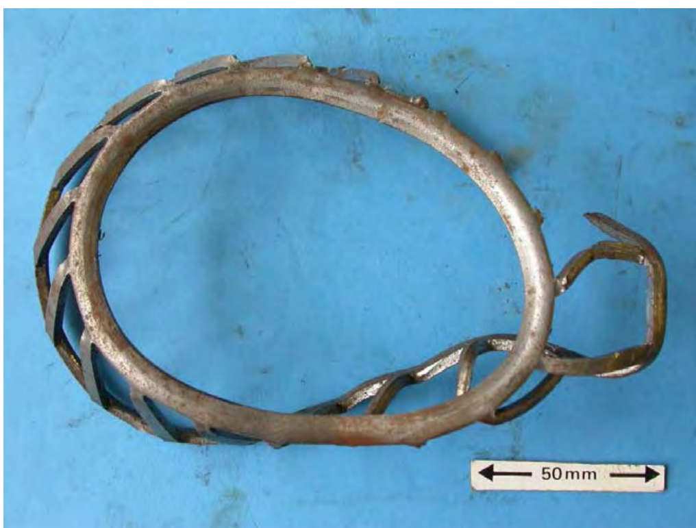
Figure 54: Roller cage from the larger of the two output shaft bearings, which exhibited evidence of post casualty damage only.
