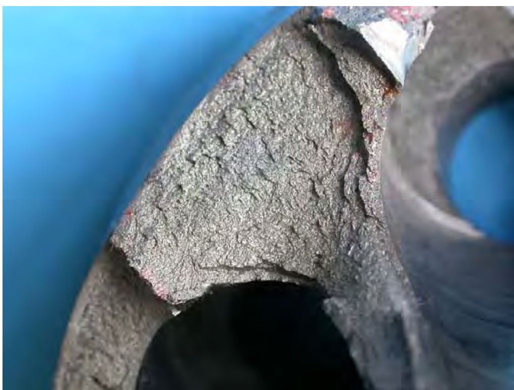
Figure 24: Third region of the cylinder block fracture surface, showing features consistent with a single event brittle fracture (post fracture mechanical damage noted).
