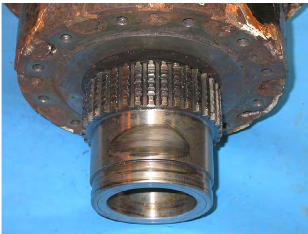
Figure 63: Output gear shafting, showing evidence of recent overheating and local seizure type damage.
