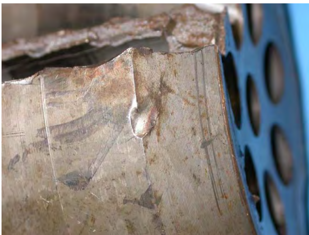
Figure 12: Typical post fracture impact damage at the cylinder clocks outer diameter.
