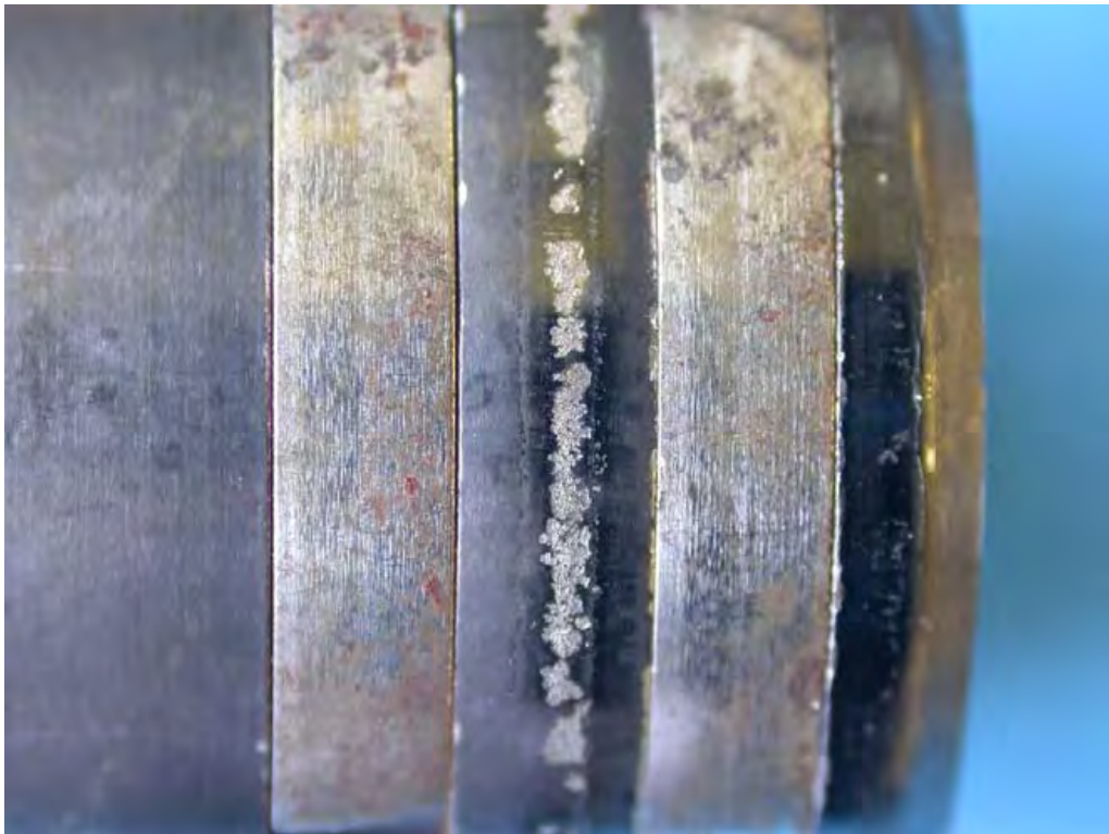
Figure 44: Detail of figure 42, showing wear or spalling of the region between the two piston rings.
