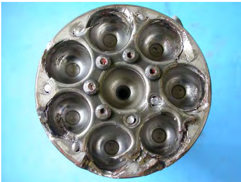
Figure 50: Output shaft pin pockets, showing evidence of local pin head seizure marks, damaged end plate and sheared cap-head studs.
