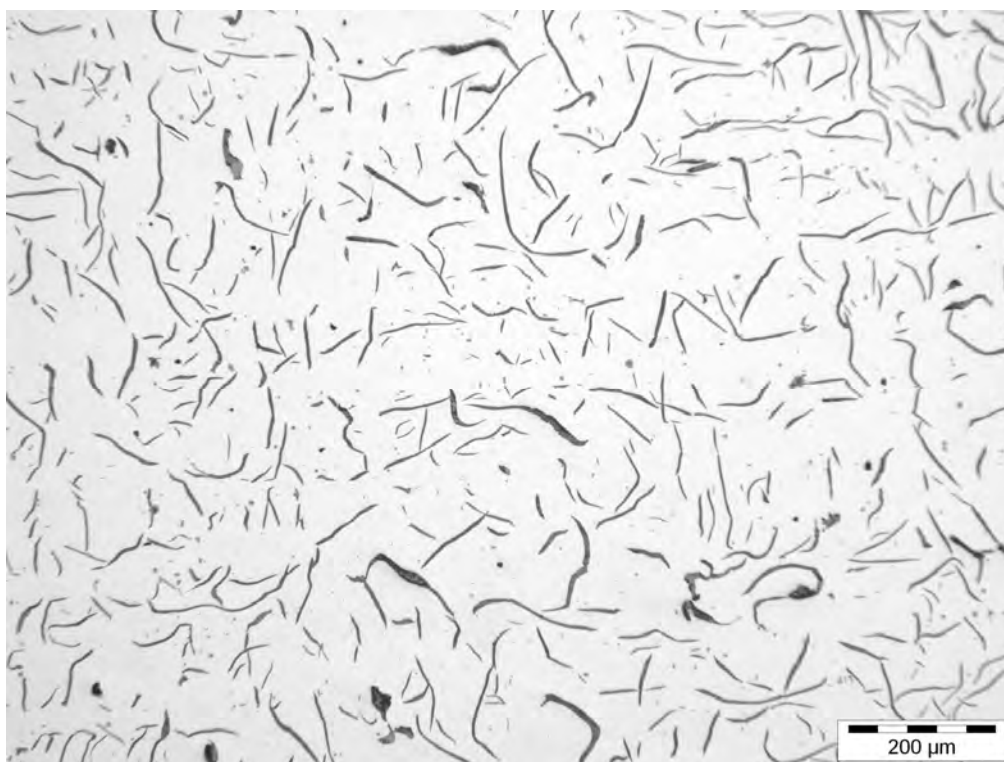
Figure 61: Micrograph (original image captured at X100), specimen unetched. Section from the fractured motor case piece illustrated in figure 58, and showing a flake graphite type morphology typical of a grey cast iron.
