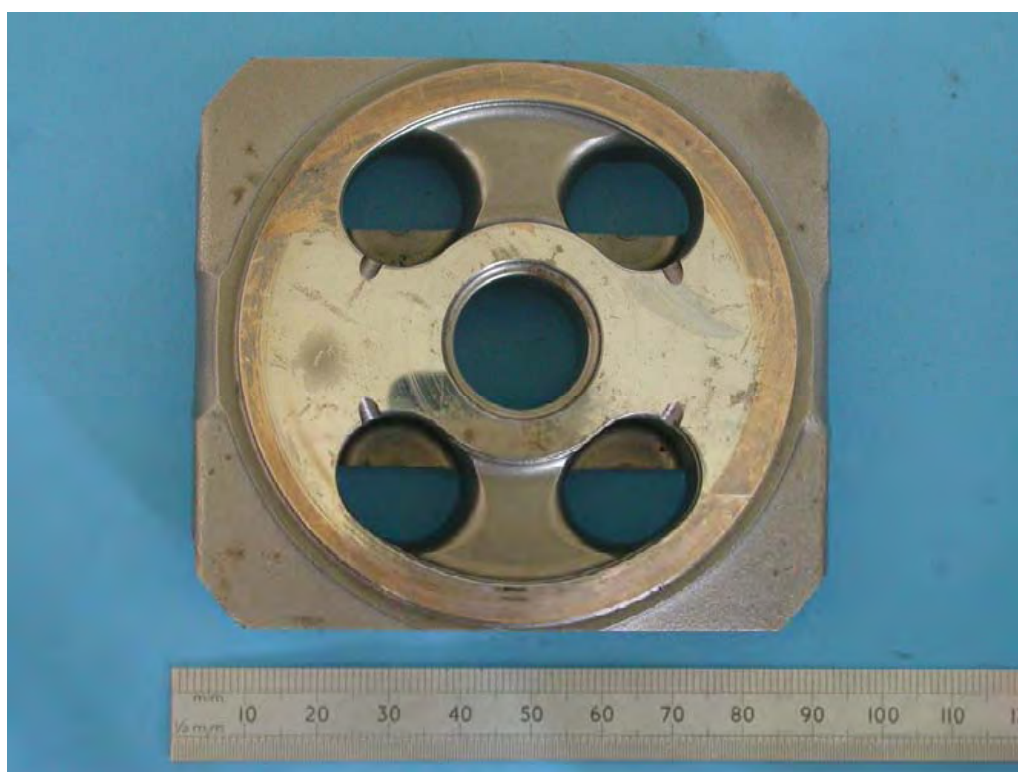
Figure 2: Cylinder block facing side of the control lens, showing evidence of only light non critical service rubbing wear.
