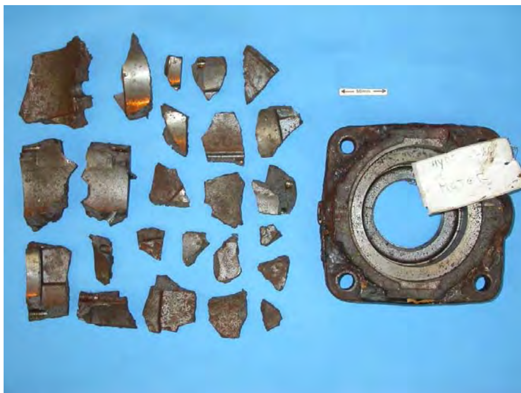
Figure 57: Recovered pieces from the extensively fractured cast iron motor casing, viewed from their opposite sides.
