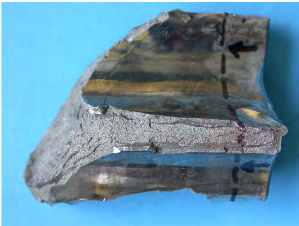
Figure 33: Detached piece from the cylinder block, showing (arrowed) the section removed for metallographic examination.
