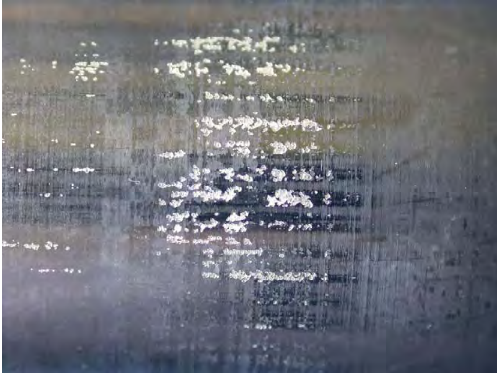
Figure 43: Detail of figure 42, showing wear or spalling of the main body region.
