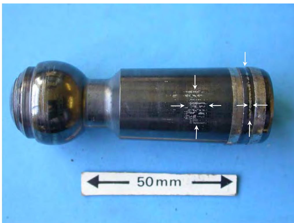
Figure 42: Incipient service wear or spalling type damage (damage sites arrowed).
