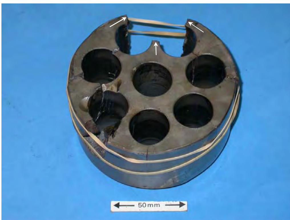
Figure 6: Fractured cylinder block, showing the location of the unrecovered fractured piece or pieces (between arrows).
