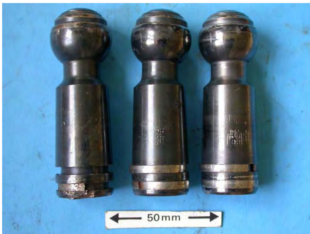
Figure 40: Three pistons recovered from the hydraulic motor and presented for laboratory examination.
