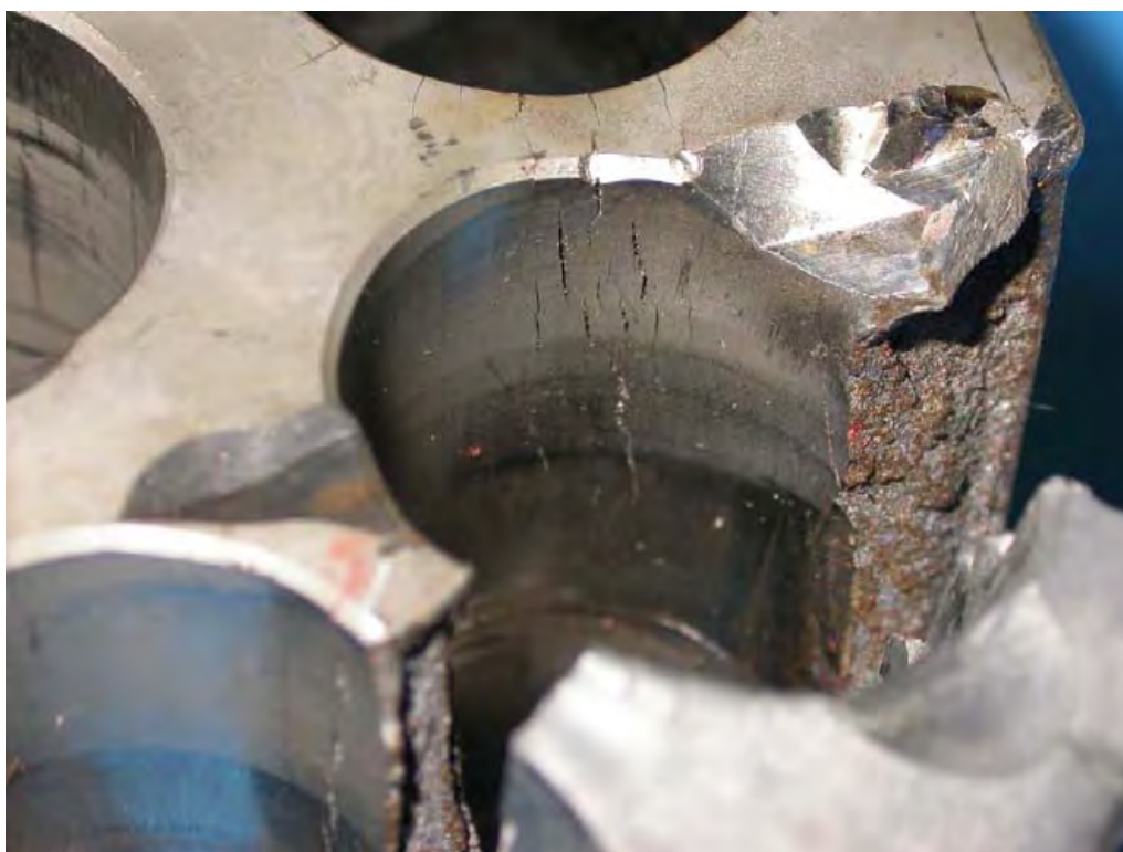
Figure 16: Secondary radial cracks, originating from the cylinder bore surface.
