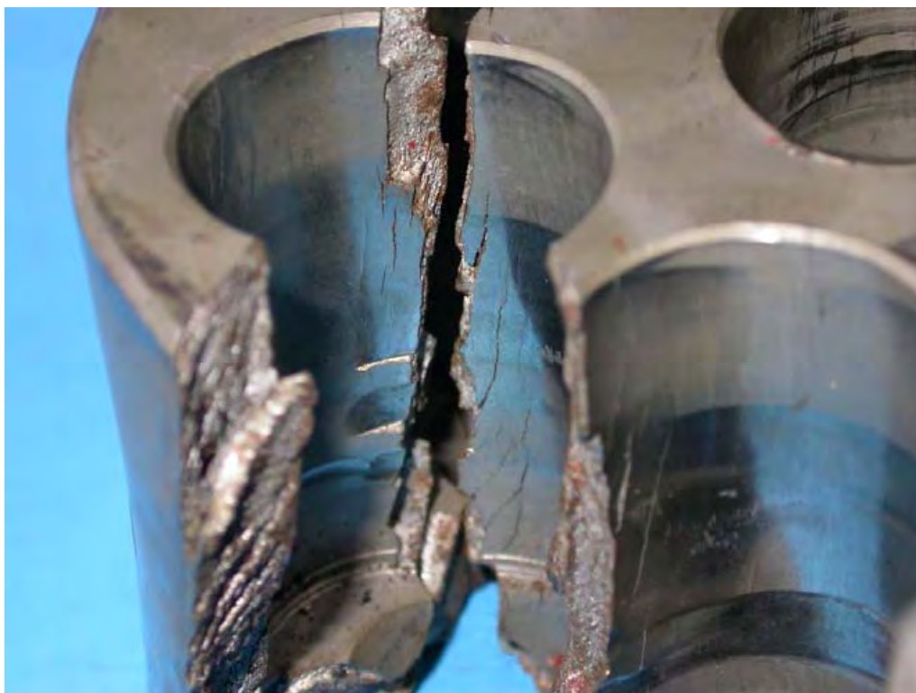
Figure 17: Detail of secondary radial cracks in two further cylinder bores.
