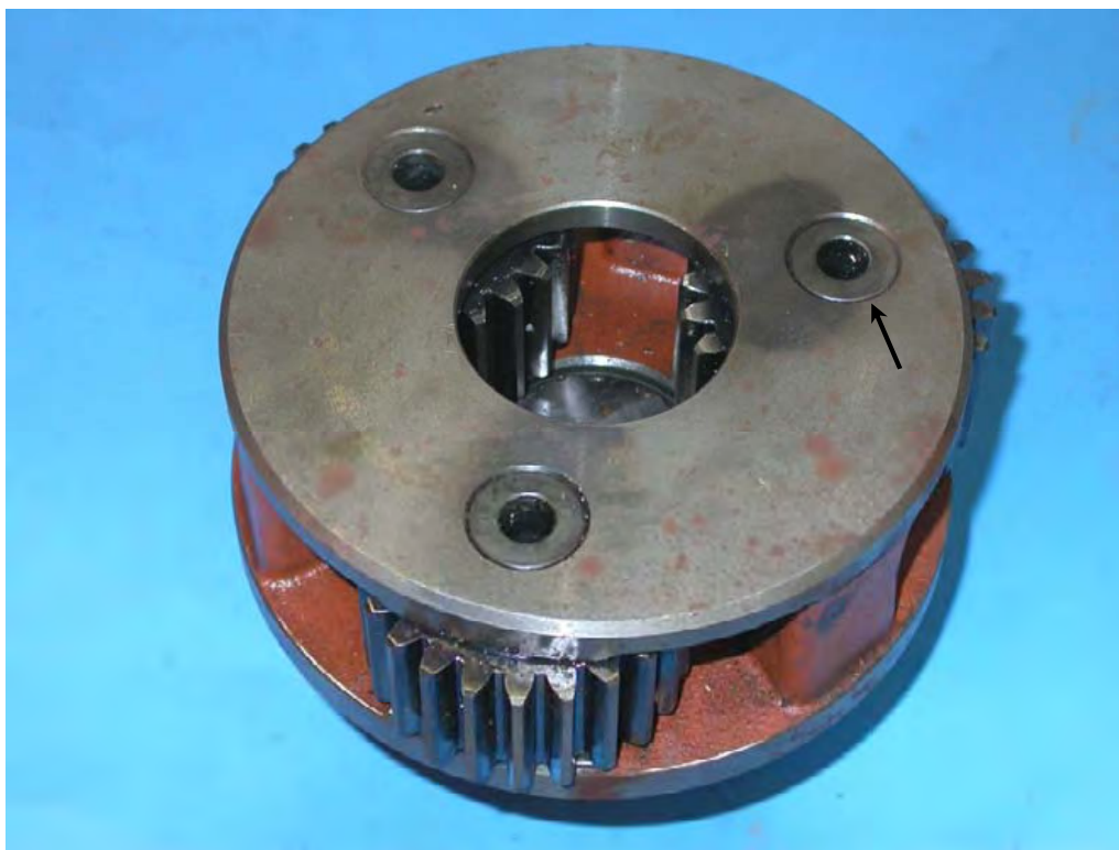
Figure 65: Planetary gear set, showing end plate bluing at the three shaft locations (seized shaft arrowed).
