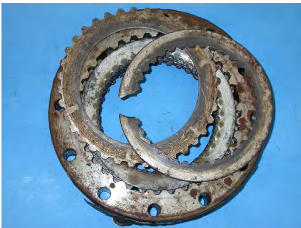
Figure 64: Recently overheated and damaged clutch/brake plate set.
