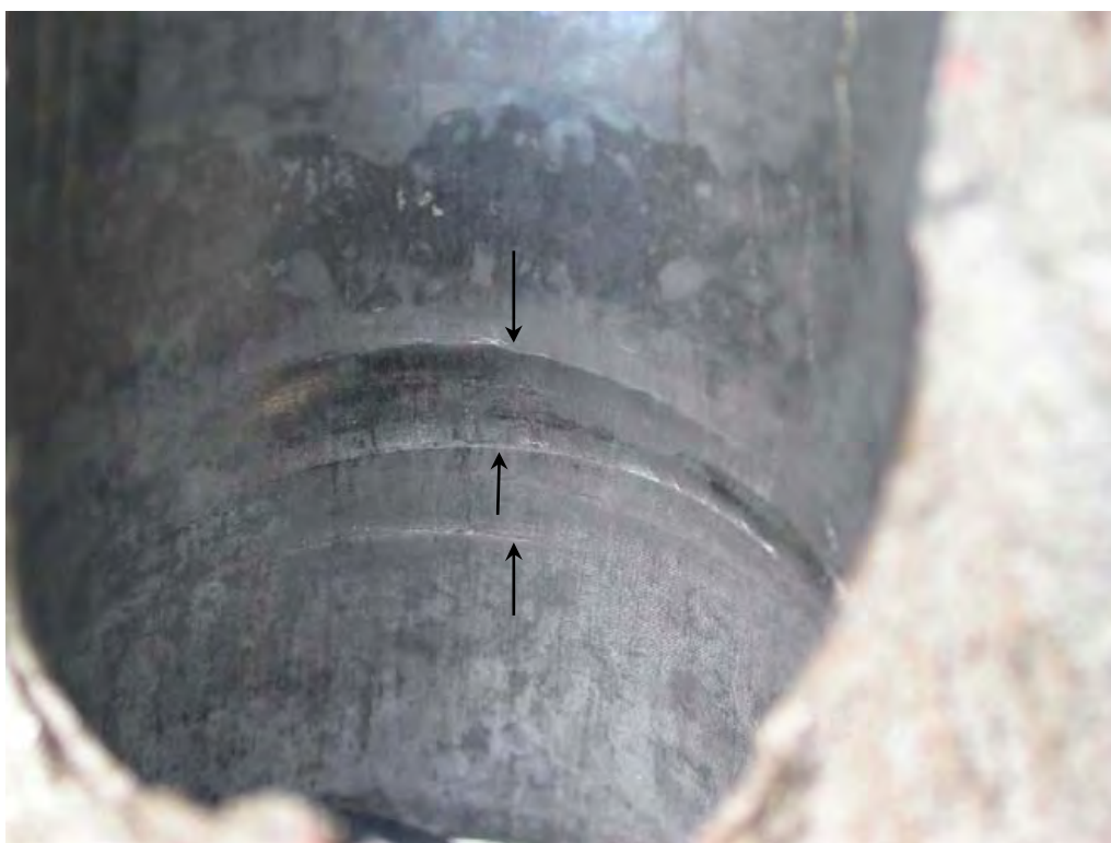
Figure 18: Piston mechanical indenting damage (arrowed) at the walls of a cylinder.
