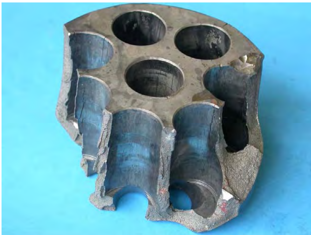
Figure 7: Largest of the recovered cylinder block pieces, showing the orientation and locations of the fracture sites (post fracture impact damage noted).
