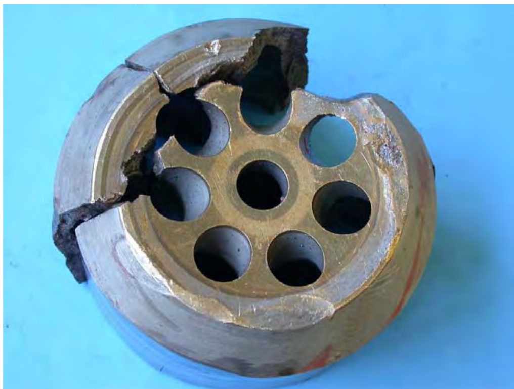
Figure 5: Fractured cylinder block, showing recovered pieces mated together and viewed from the control lens mating face.
