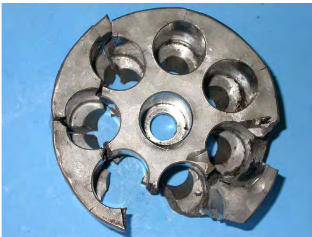
Figure 13: Secondary radial cracks, which were apparent at the cylinder blocks output end.
