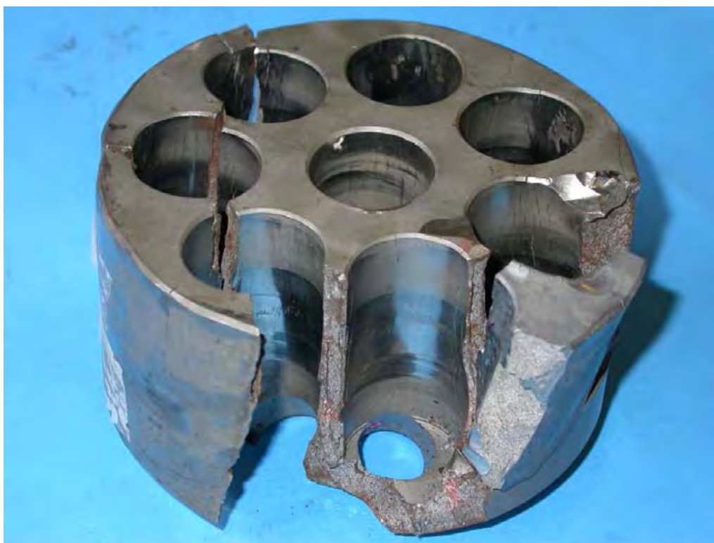
Figure 3: Fractured cylinder block, showing recovered pieces mated together.
