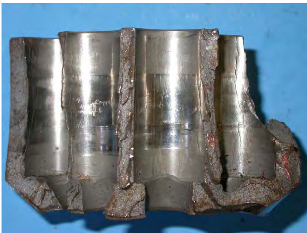
Figure 8: Second of the recovered cylinder block pieces, showing the orientation and locations of the fracture sites (post fracture impact damage noted).
