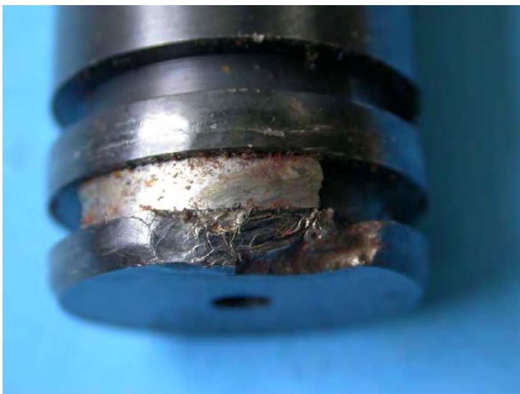
Figure 41: Piston crown end, showing loss of one and a half piston rings and associated local post fracture damage to the crown end.
