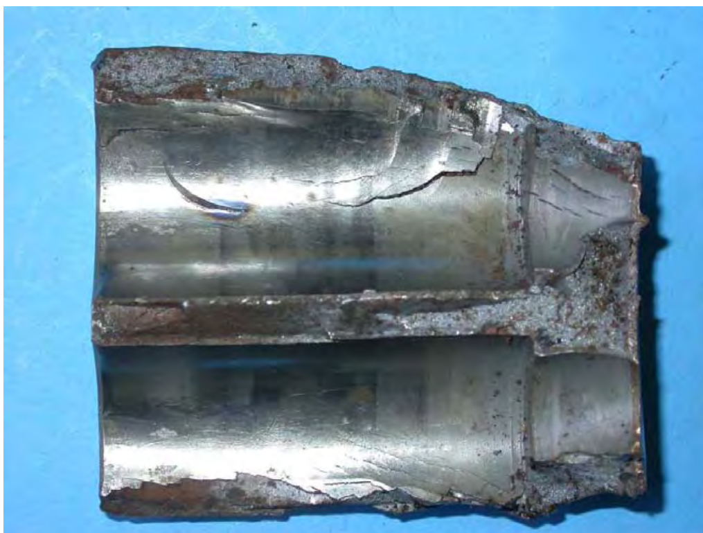
Figure 10: Fourth of the recovered cylinder block pieces, showing the orientation and locations of the fracture sites (post fracture impact damage noted).
