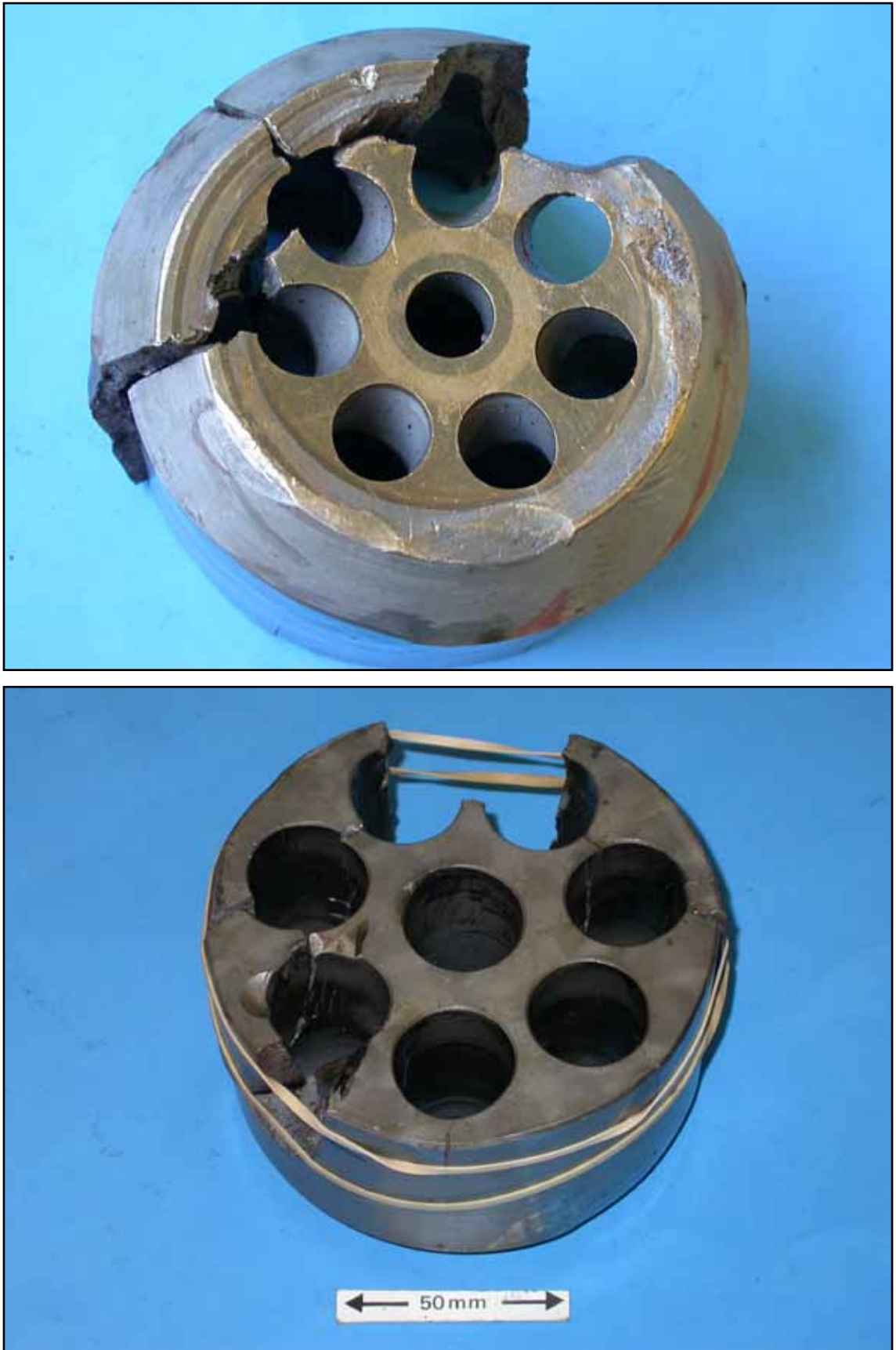
Predominant damage on one side of the cylinder housing
