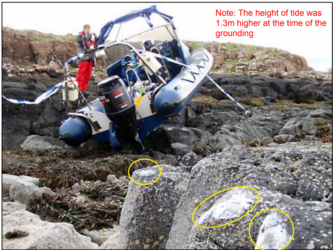
Evidence of gel coat to starboard
