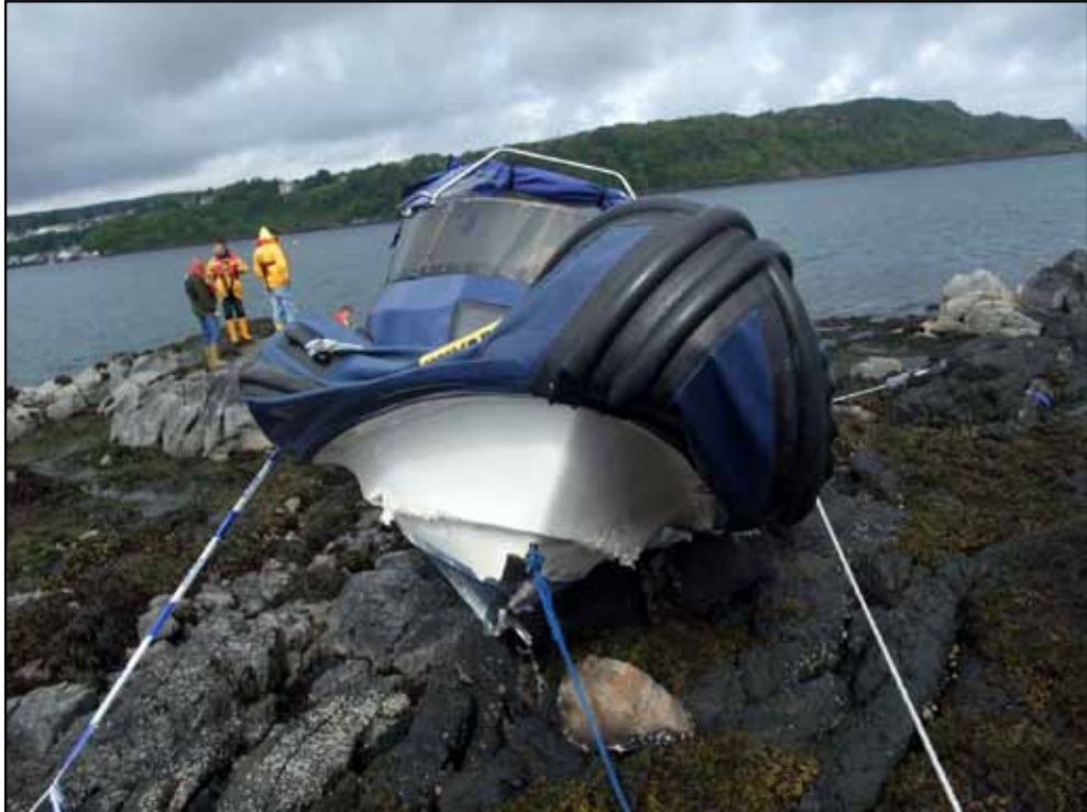
Damage to hull and forward buoyancy tube
