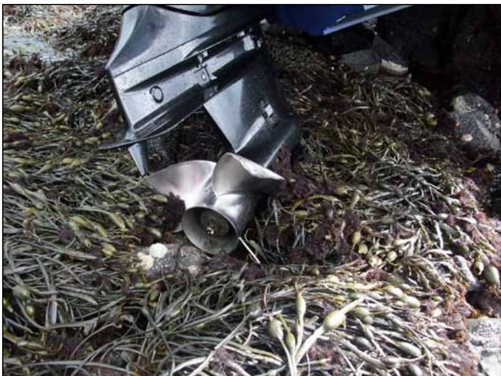
Damage to propeller blades
