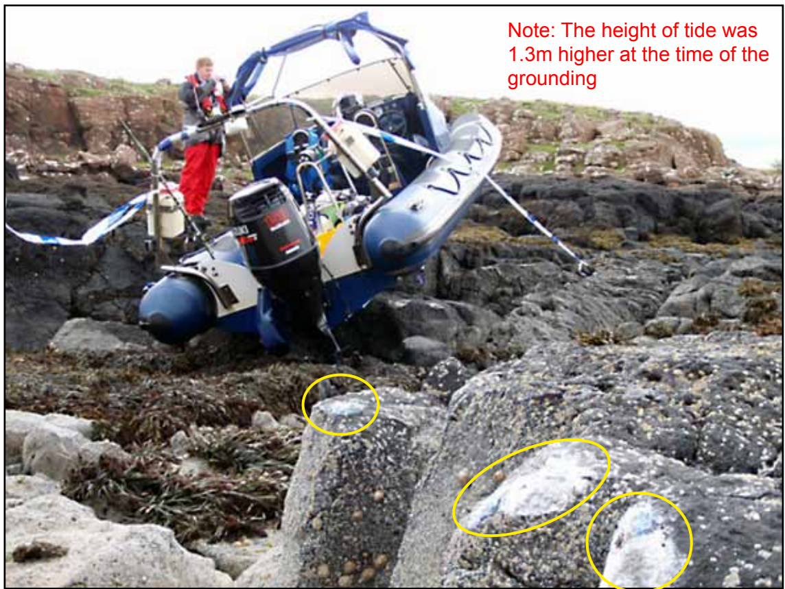
Evidence of gel coat to starboard
