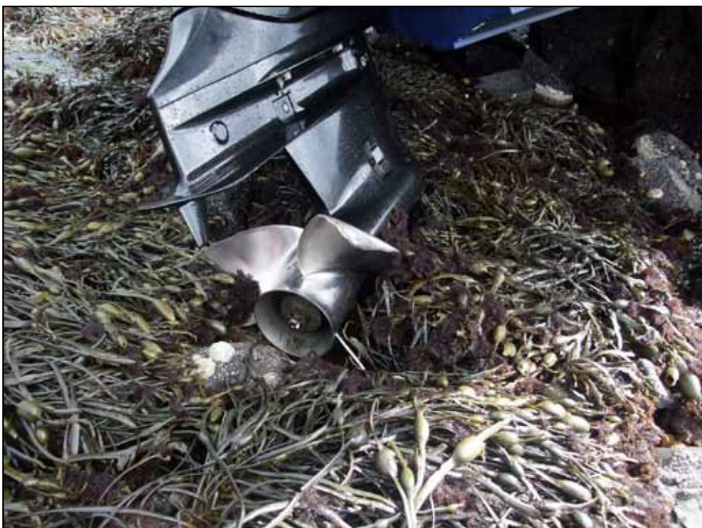
Damage to propeller blades
