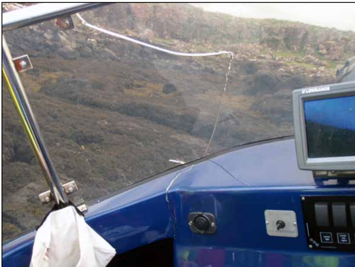
Damage to tinted visor and the console
