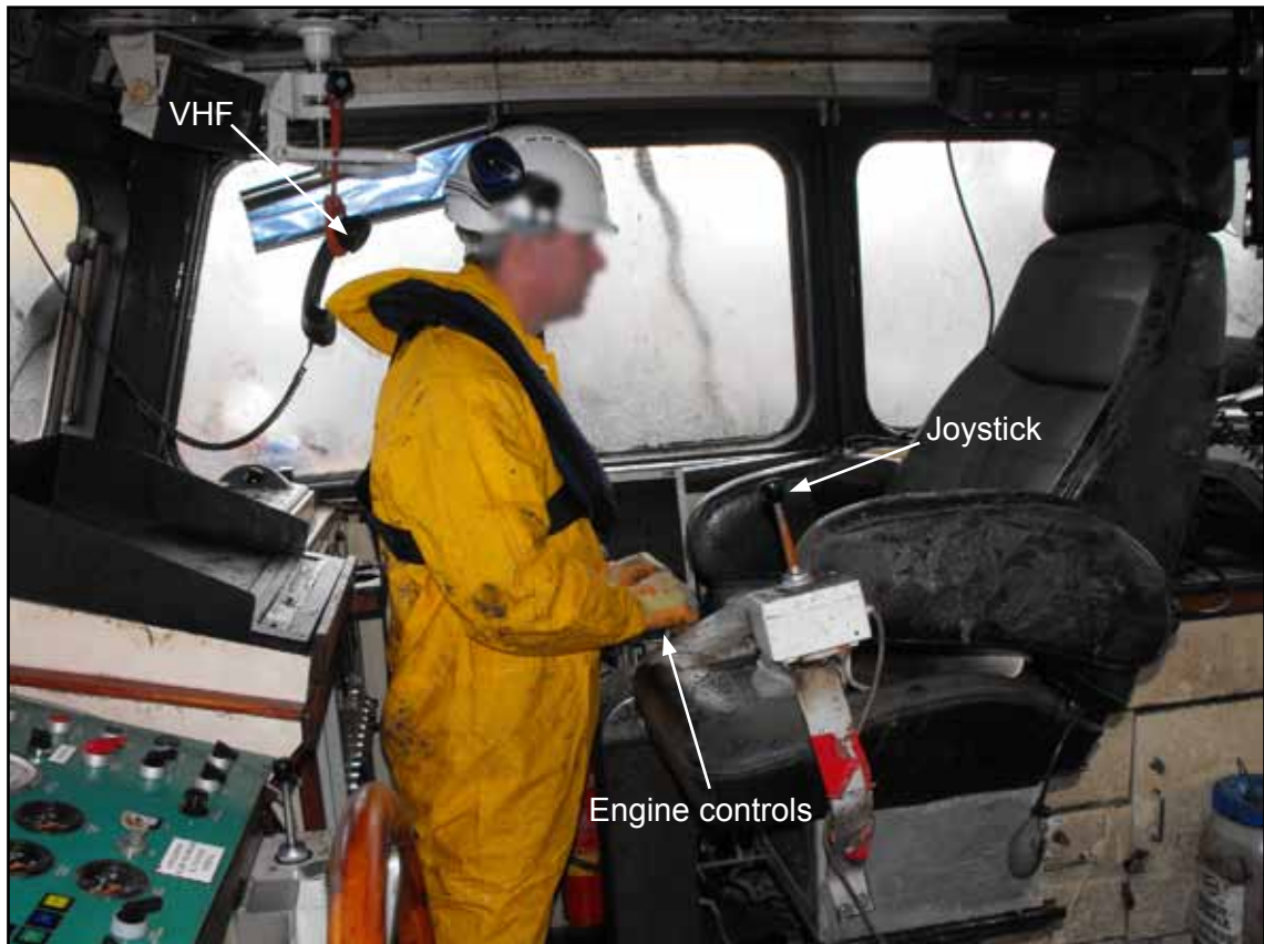
Conning position showing skipper's chair facing forward
