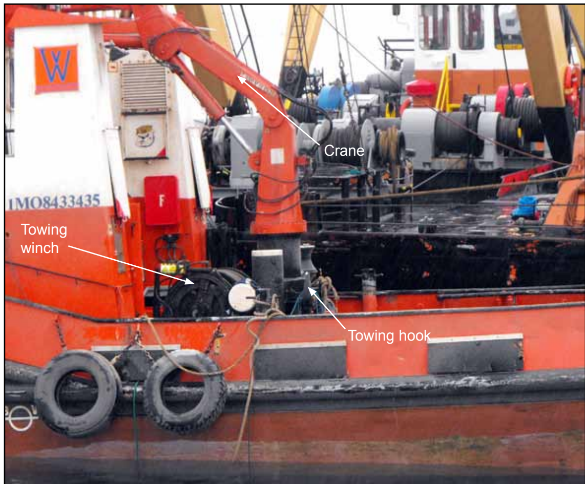
Ijsselstroom aft deck gear
