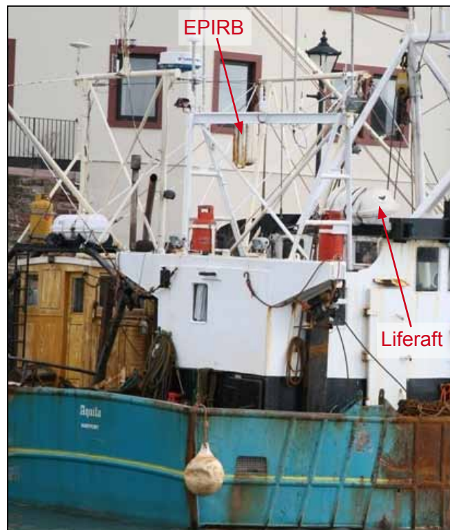
EPIRB and liferaft stowage positions on Aquila
