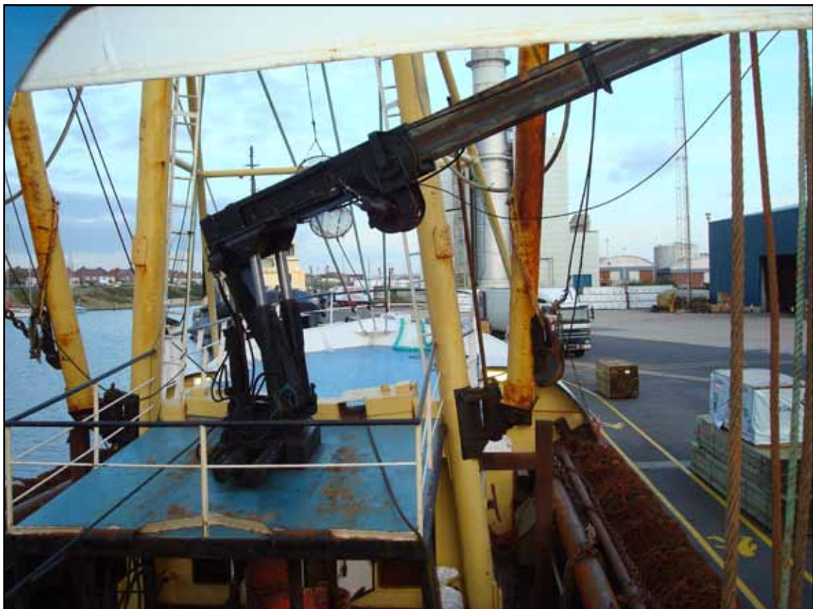
Additional HIAB crane fitted in 2009
