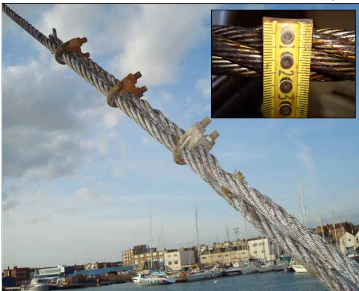
Main trawl wire (Bulldog grips incorrectly rigged)
