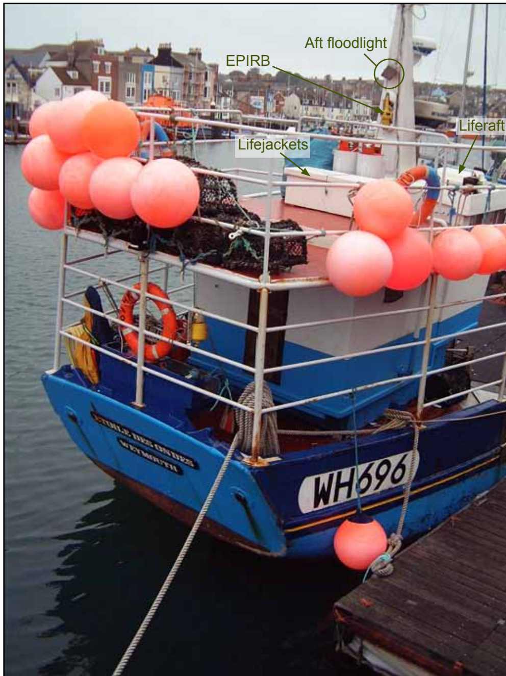
General overview of Etoile des Ondes ' wheelhouse top and quarter deck (deck shelter omitted for clarity)
