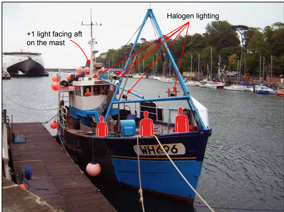
Etoile des Ondes - with halogen lighting and crew positions indicated (whaleback omitted for clarity)
