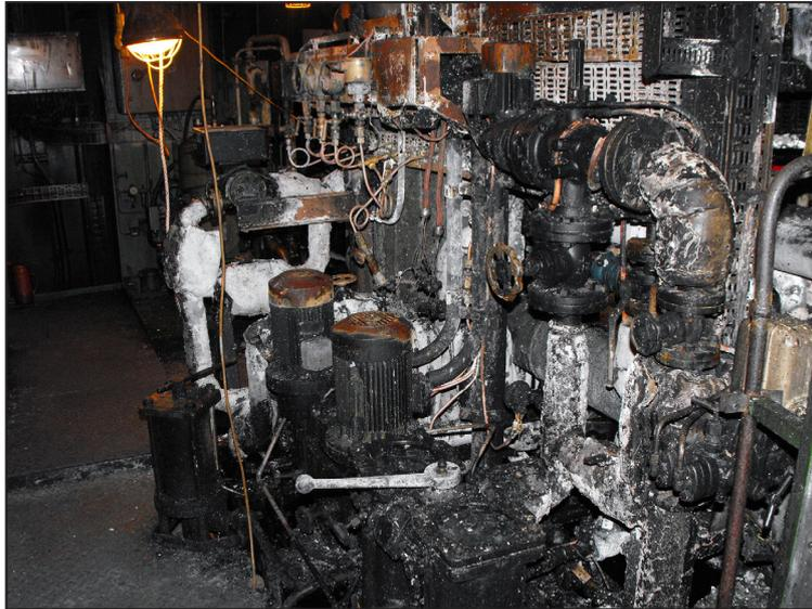
As part of the fire-fighting effort, the fixed total flooding system (high expansion foam) was activated but did not extinguish the fire. Although all of the foam solution in the system was deployed into the auxiliary engine room, no foam was produced. The fire burned fiercely for over 1 hour before it was extinguished by the ship's crew.
