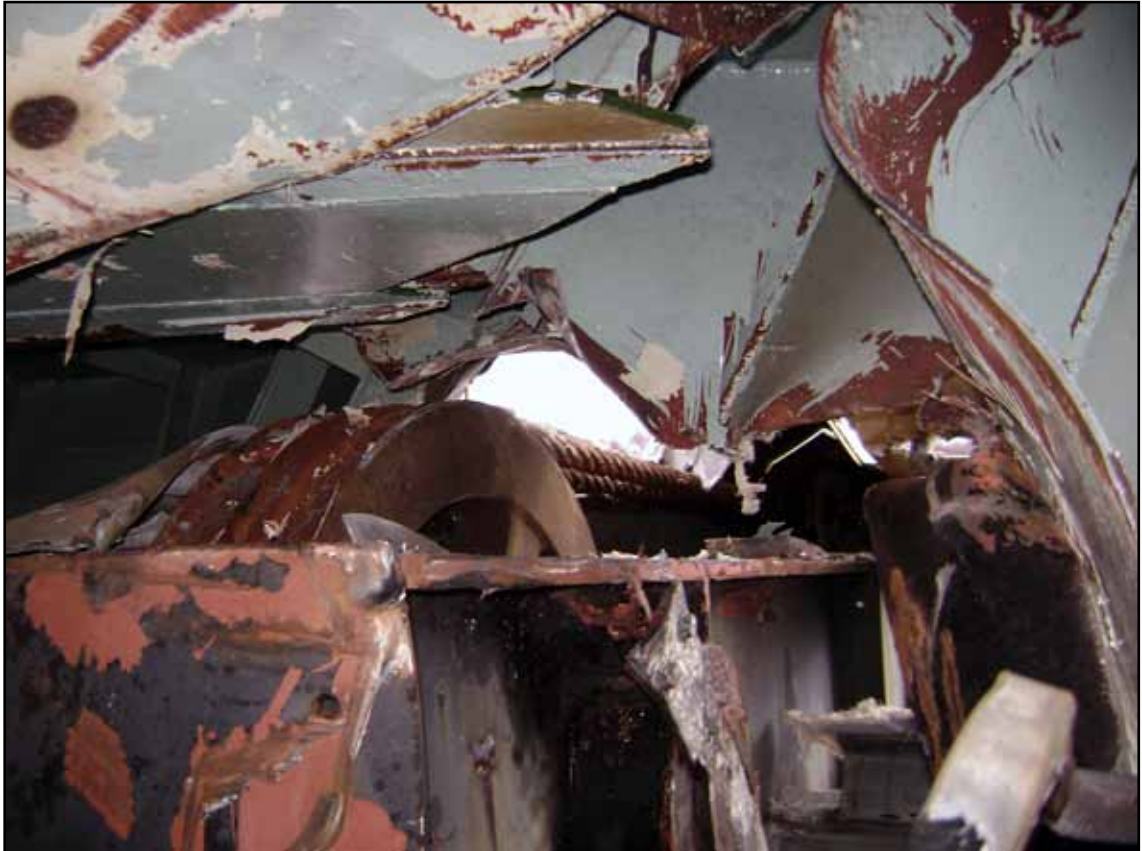
Linkspan arm penetration of bow visor
