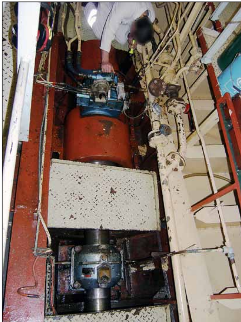
Starboard CPP OD box and propeller shaft
