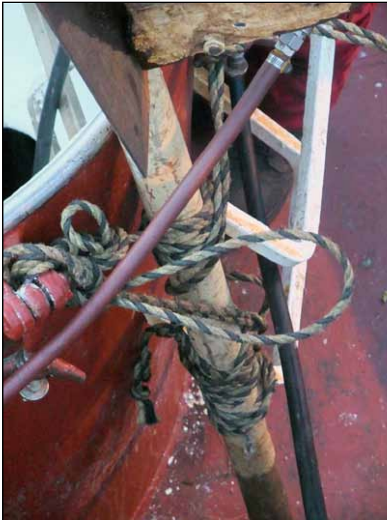
Casualty rescue equipment securing arrangements to No 2 cargo tank hatch coaming
