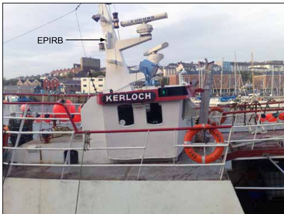
Photograph of Kerloch showing EPIRB mounted on mast
