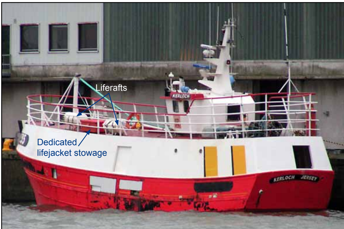
Photograph of Kerloch showing liferafts and dedicated lifejacket stowage
