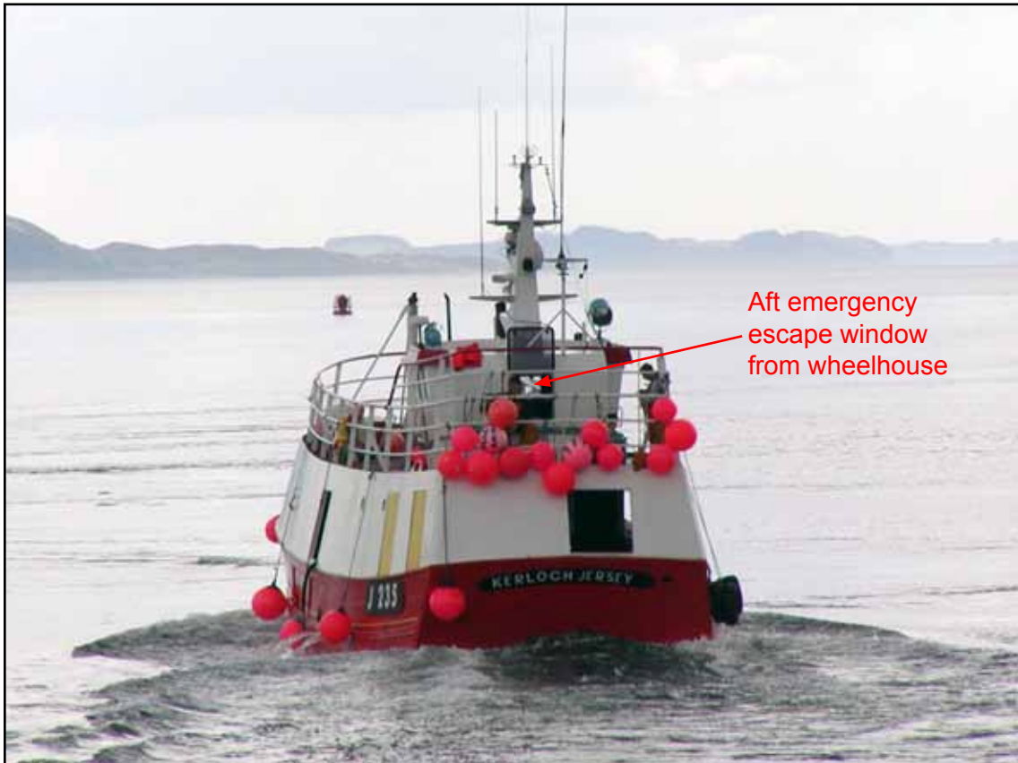
Photograph of Kerloch showing aft emergency escape window
