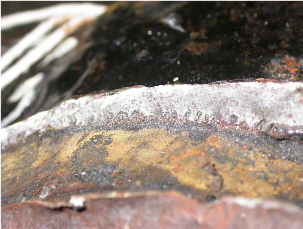
Figure 7: Sheared starboard ring retaining fillet weld, showing root worm-hole porosity.
