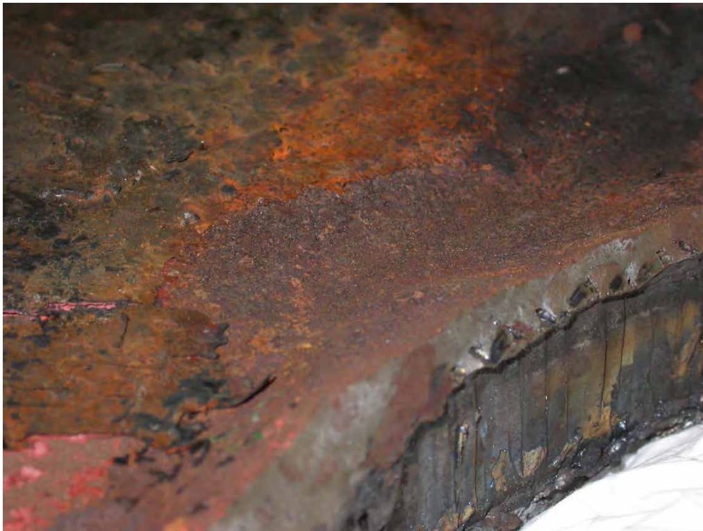
Figure 13: Port side plate, showing local corrosion wastage apparent at one of the plate faces adjacent to the fracture site.
