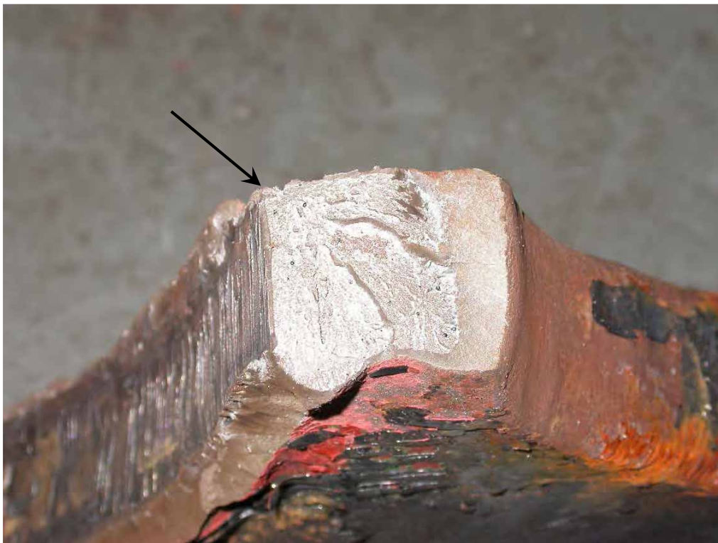
Figure 2: Second fracture in the starboard plate (fracture origin shown arrowed).
