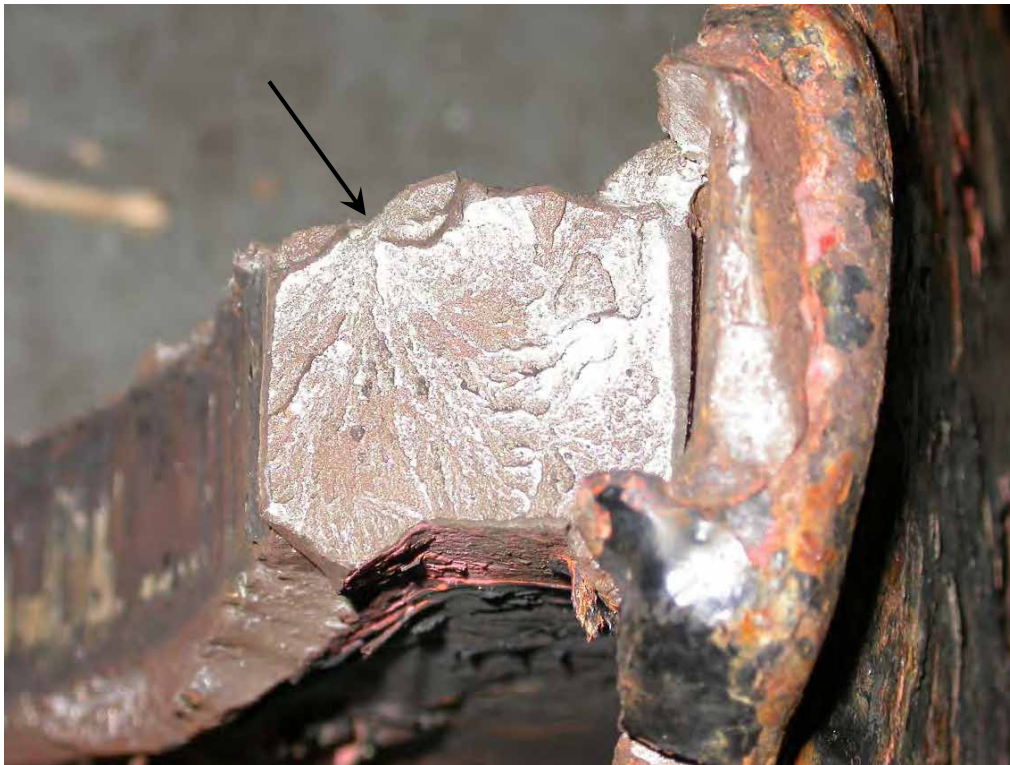
Figure 9: Fracture in the port plate (fracture origin shown arrowed).
