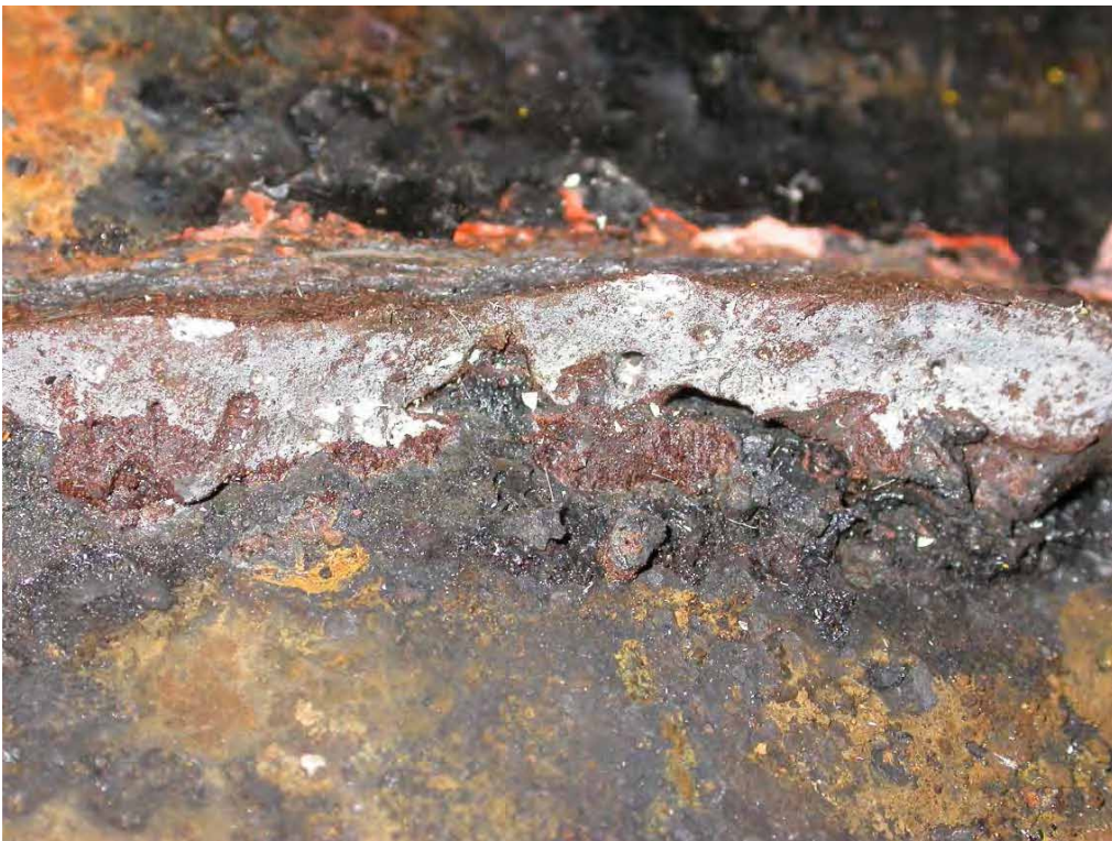
Figure 8: Sheared starboard ring retaining fillet weld, showing local lack of fusion.
