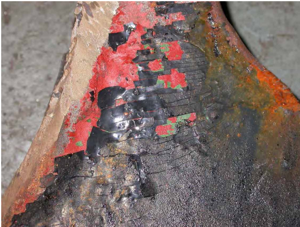
Figure 3: Evidence of post yield point type straining (as evidenced by cracking in the paint) for a considerable distance back from the starboard side fracture site.
