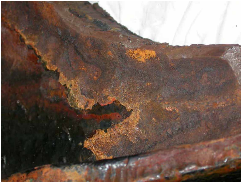
Figure 5: Starboard side plate, showing local corrosion wastage apparent at one of the plate faces adjacent to the fracture site.
