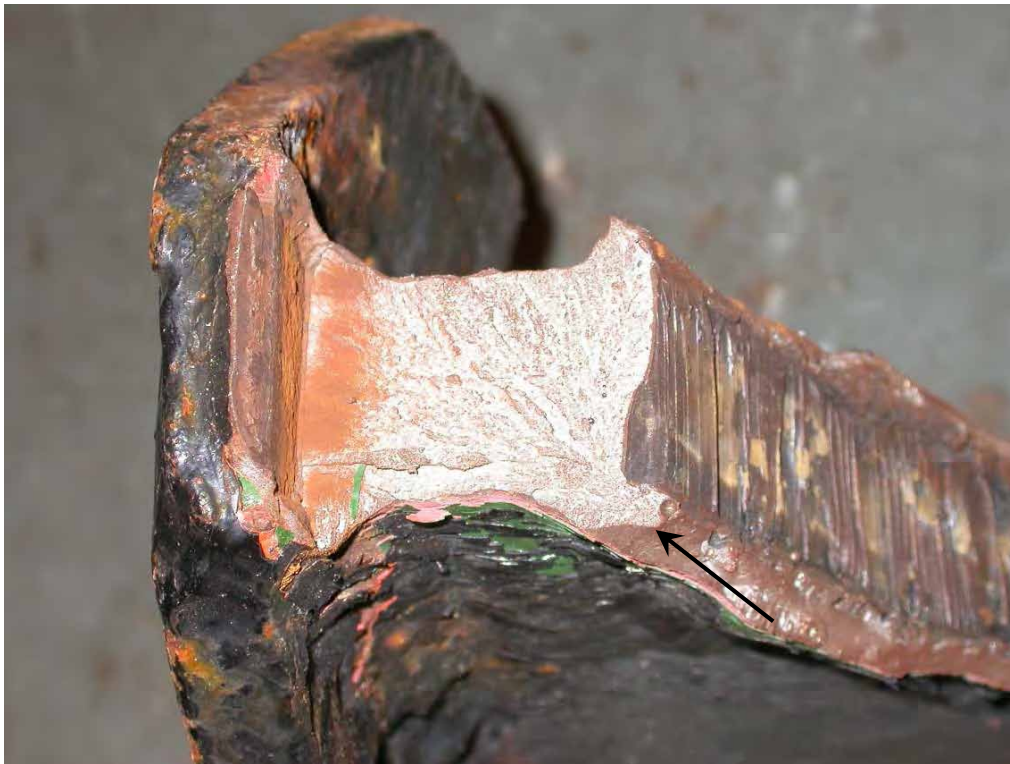
Figure 1: Fracture in the starboard plate (fracture origin shown arrowed).
