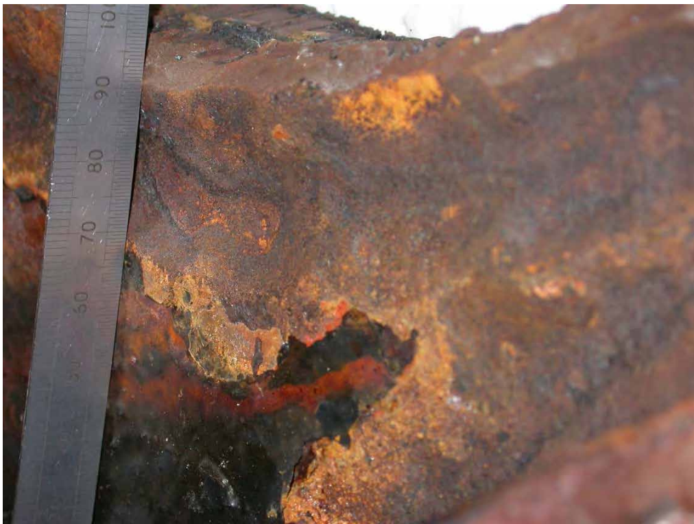
Figure 6: Detail of local corrosion wastage shown in figure 5.
