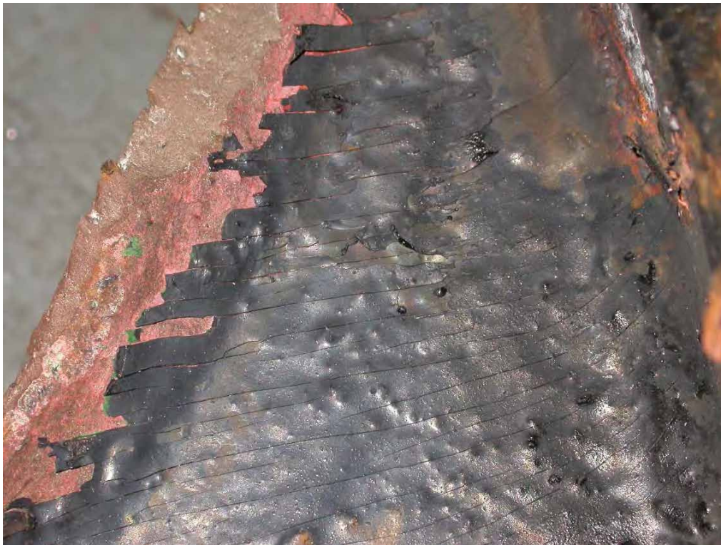
Figure 11: Evidence of post yield point type straining (as evidenced by cracking in the paint) for a considerable distance back from the port side fracture site.
