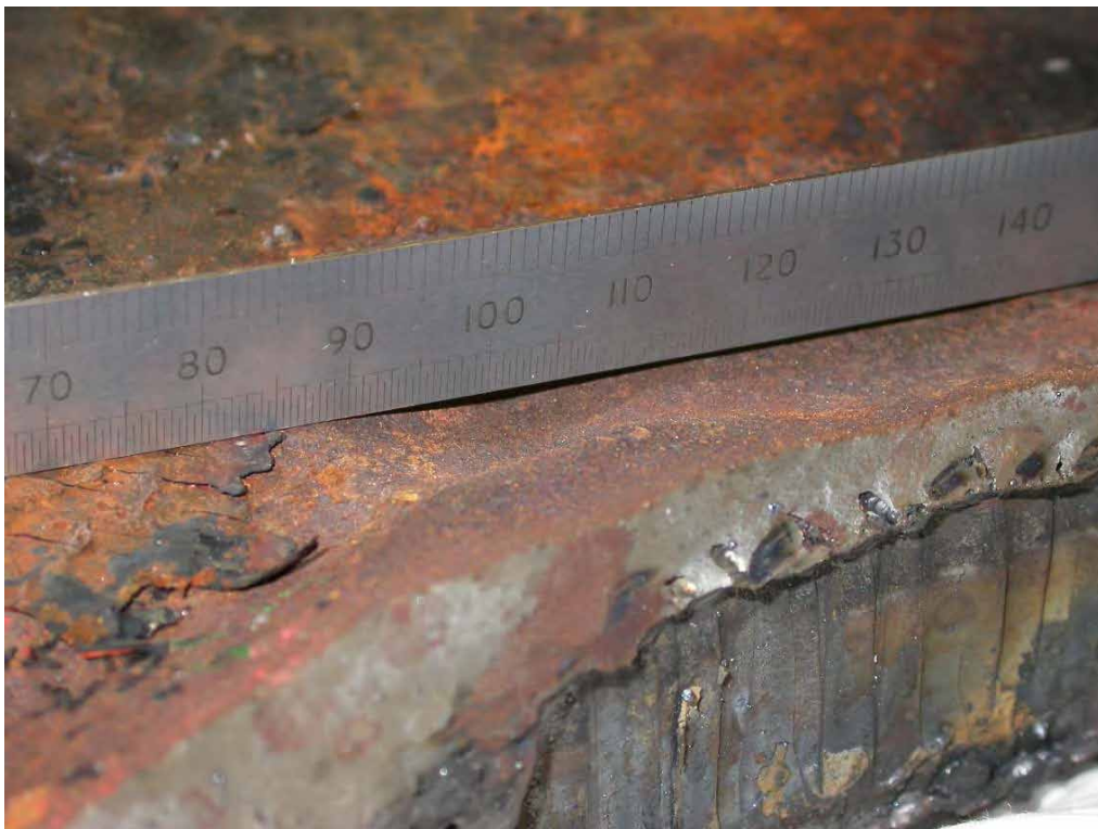
Figure 14: Detail of local corrosion wastage shown in figure 13.
