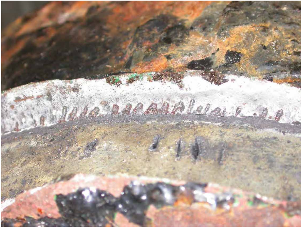
Figure 15: Sheared port ring retaining fillet weld, showing root worm-hole porosity.
