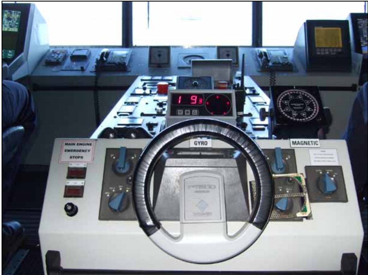
Centre control panel (bridge), looking forward
