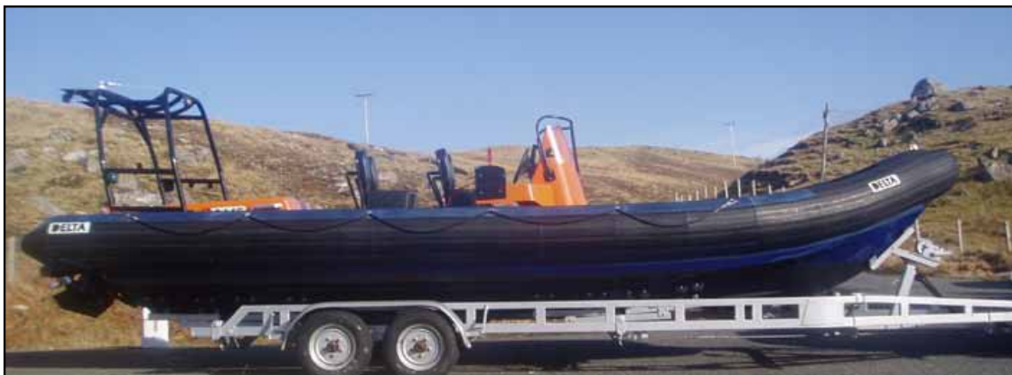
The Delta 8.5m RIB on its launching trailer
