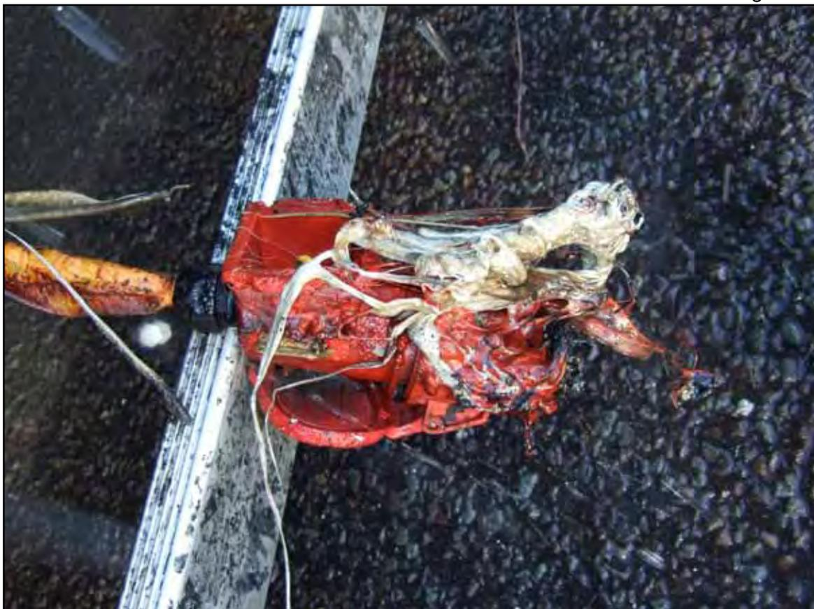
Damaged external power supply connection on trailer CRF459
