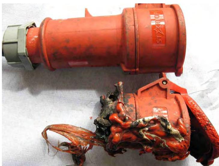
**Figure 15** Damaged and undamaged free socket
