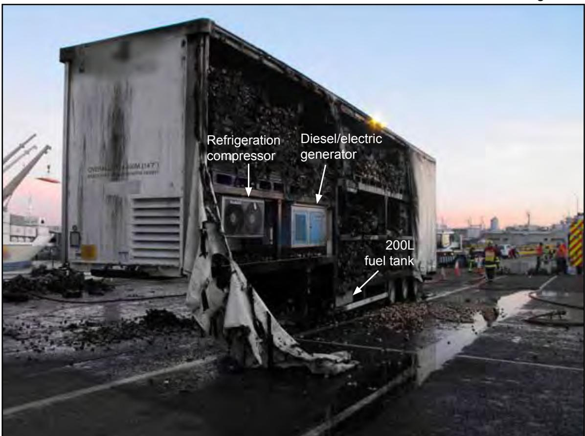
Diesel generator, refrigeration compressor and fuel tank
