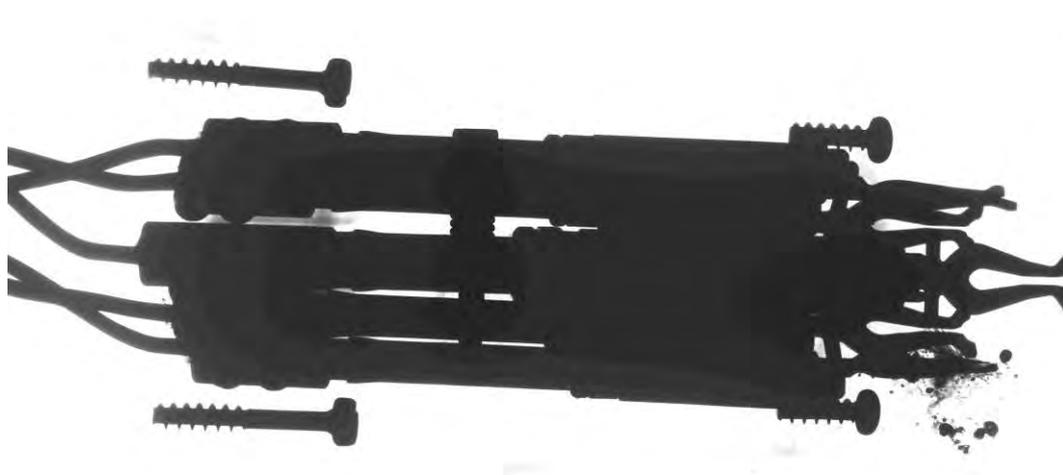
**Figure 7 X-ray of plug and socket**
