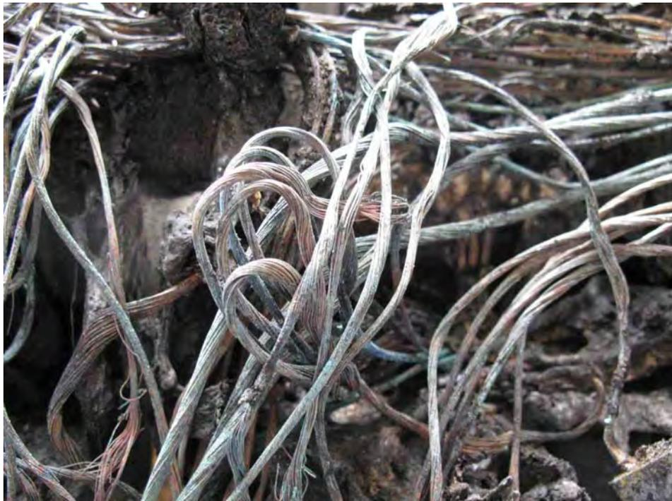
**Figure 11** Fire damaged wiring
