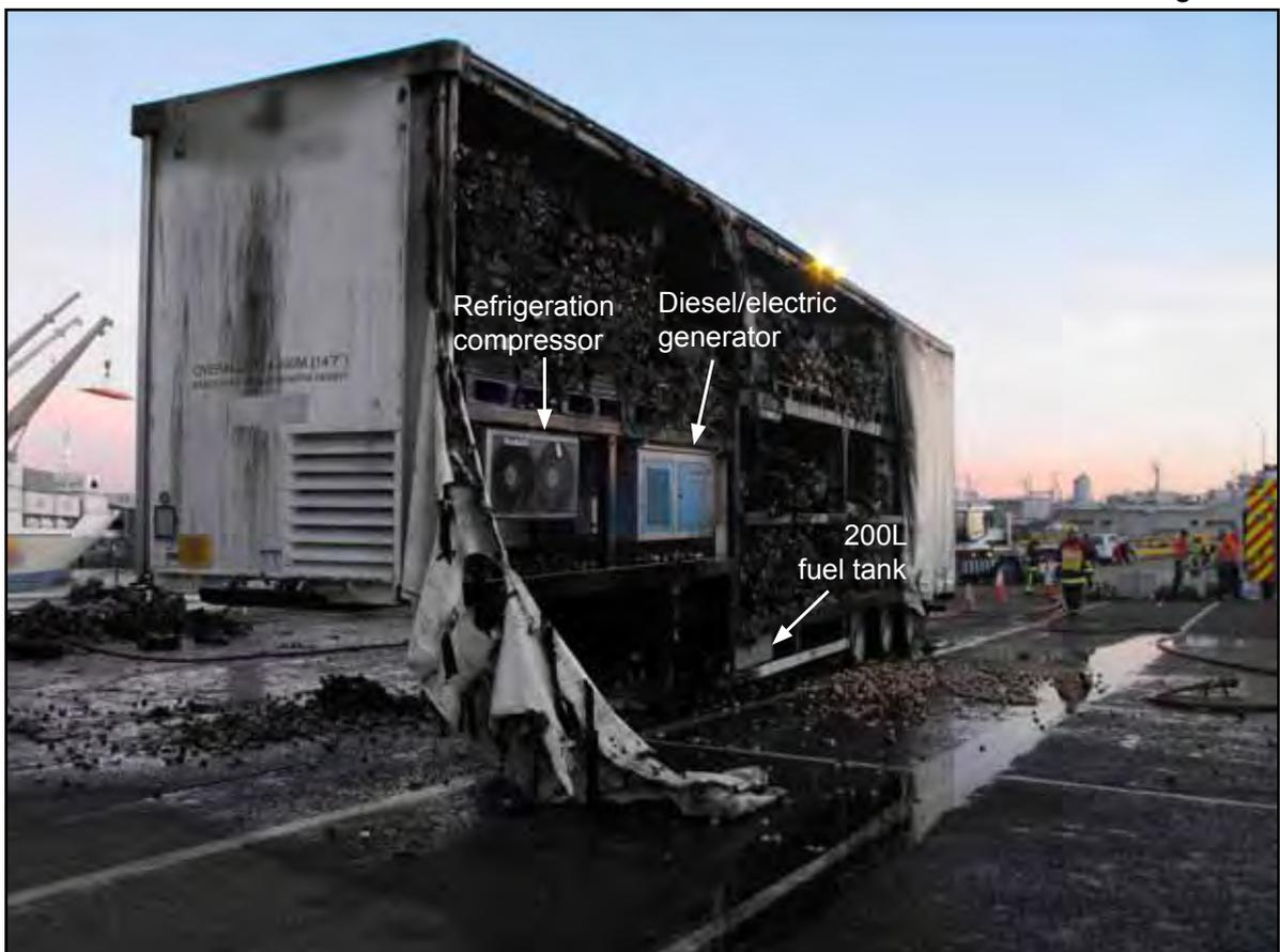
Diesel generator, refrigeration compressor and fuel tank
