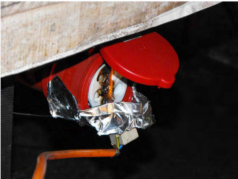
**Figure 5 Initial flaming of plastic core**
