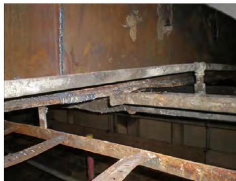
Frame 77, web and lower flange buckled (buckled longitudinal deep frame already removed)
