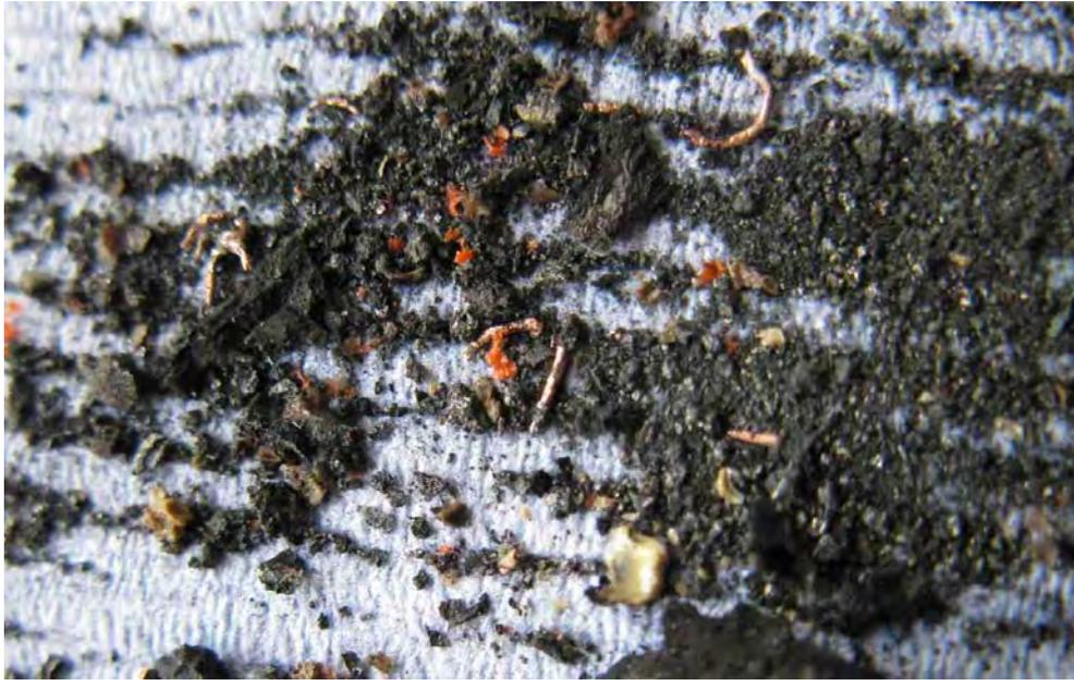
**Figure 22** Conductor strands and copper globules
