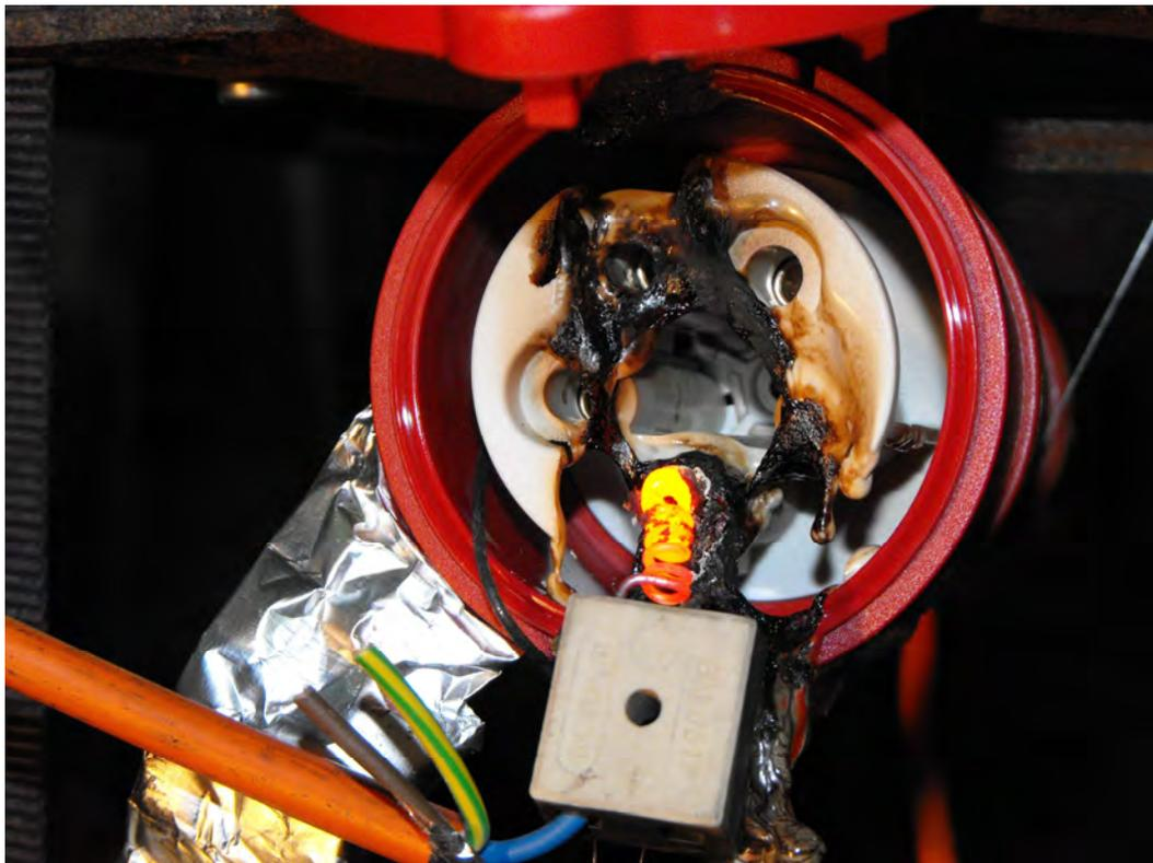
**Figure 6 Damage to socket from initial flaming**
