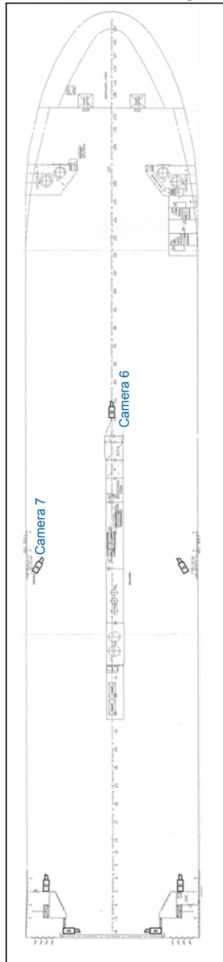
Layout of CCTV cameras on the main vehicle deck
