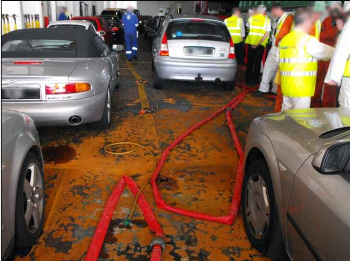
Heat damage to the upper vehicle deck
