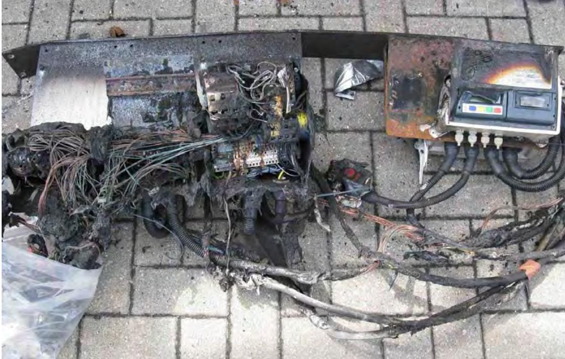
**Figure 4** Control box assembly, fire damaged
