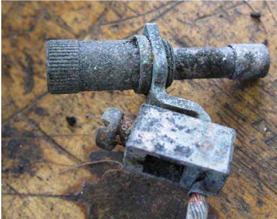
**Figure 12** Terminal and spring contact
