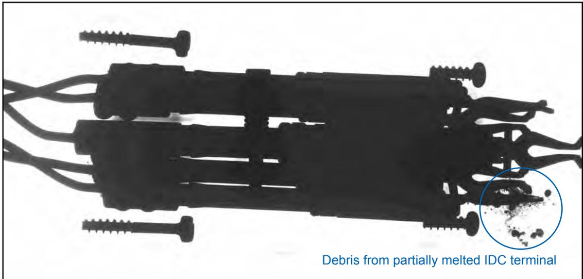
X-ray of the external power supply connection on trailer CRF459
