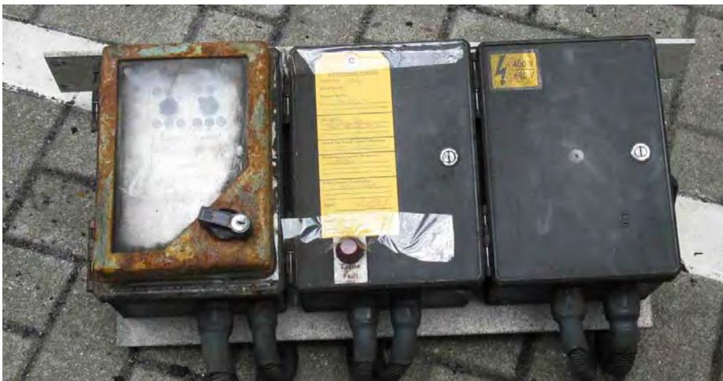
**Figure 5** Control box assembly, undamaged
