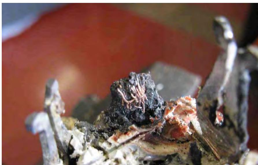
**Figure 21** Conductor strands adhered to terminal
