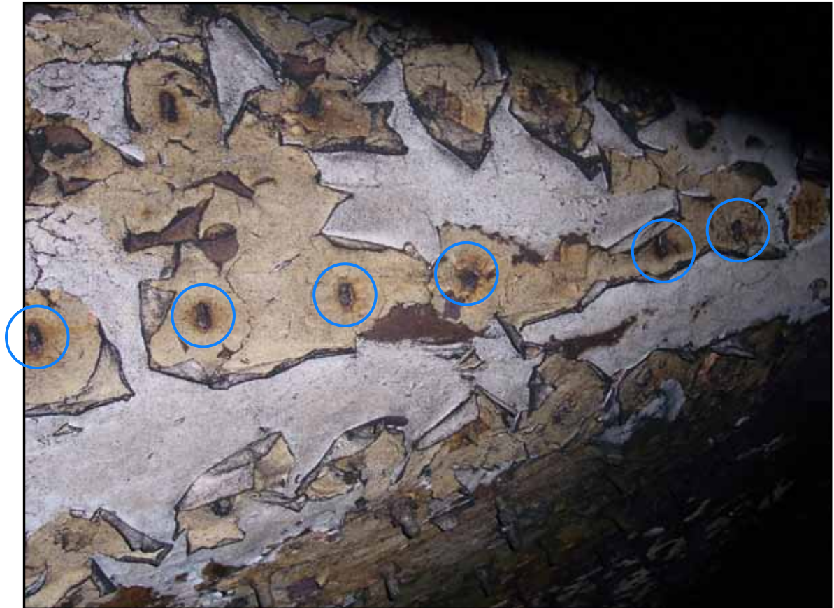
Elongation of hopper carcass "Hardox" tile securing stud holes
