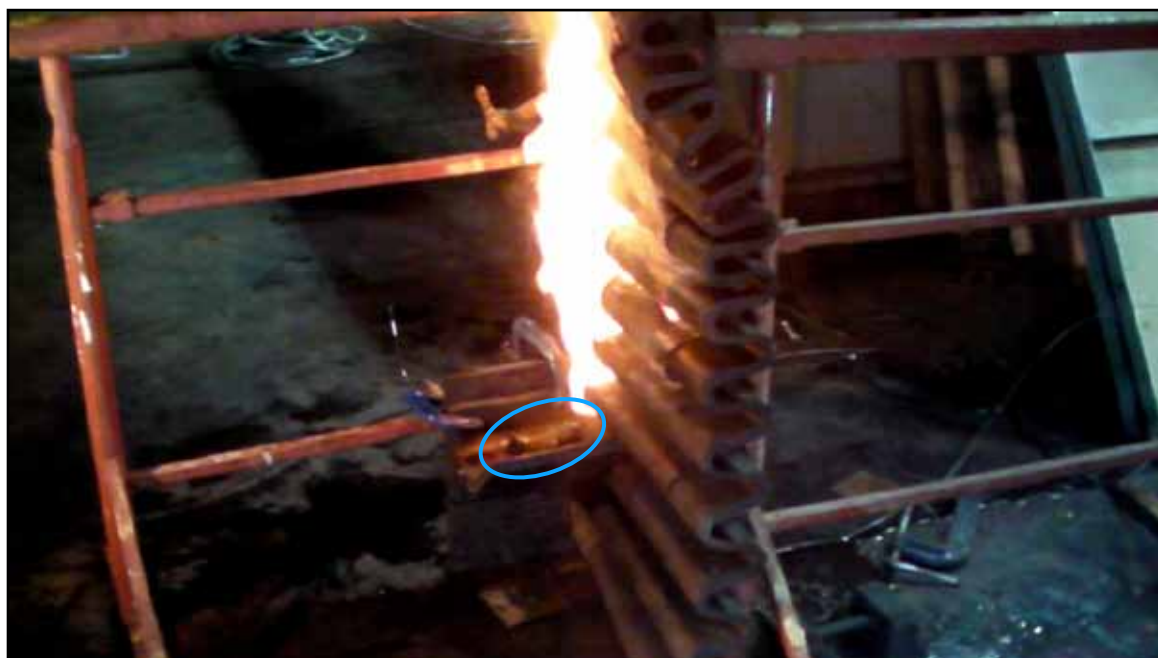
Fire Tests - stud and nut placed in cleat adjacent to the side curtain after 10 minutes
