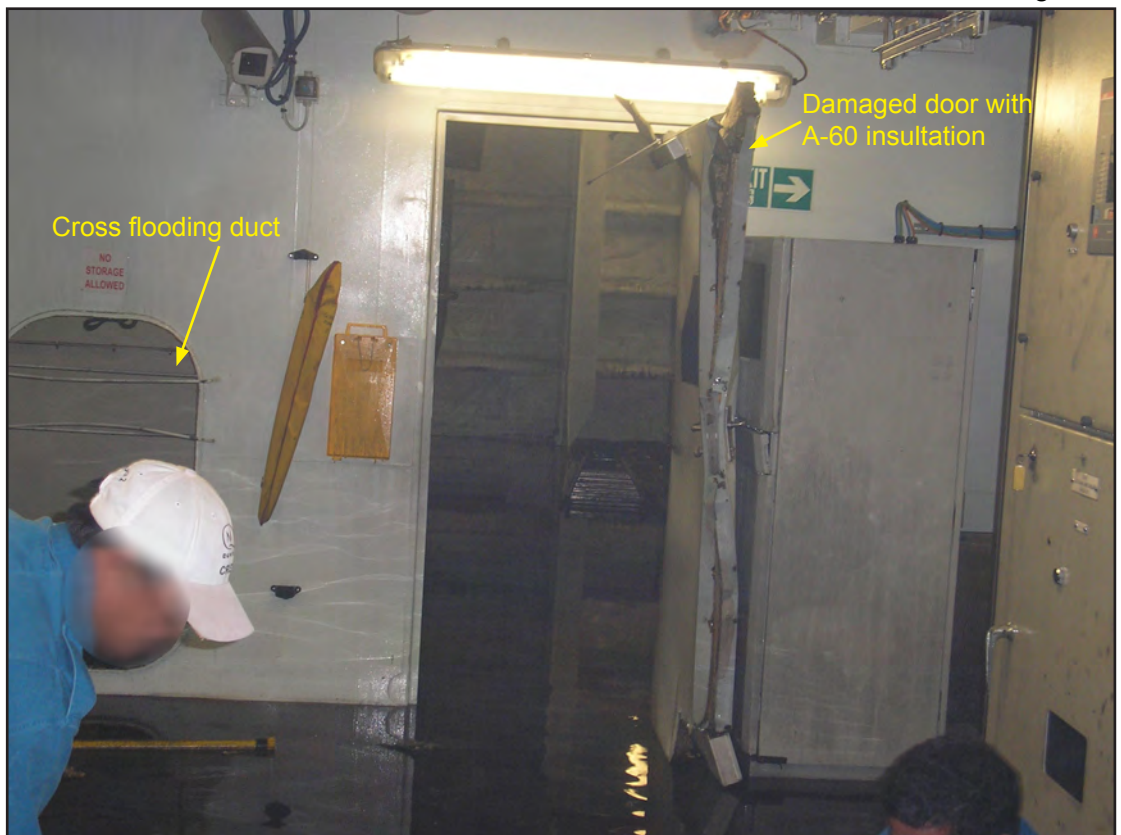
Water in the aft harmonic filter and main switchboard rooms
