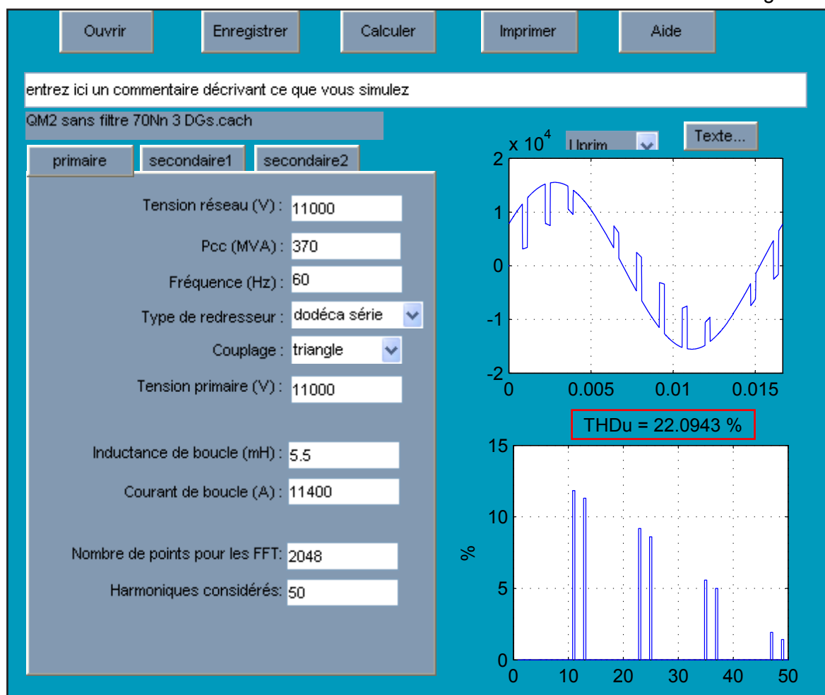
Simulation of expected total harmonic distortion of voltage with three diesel generators and at 70% propulsion power output
