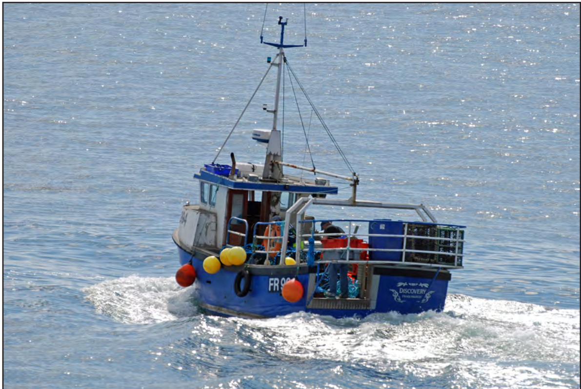
Discovery showing closable stern door arrangement
