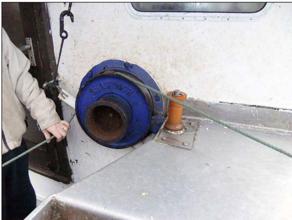
Back rope led to hauler without using vertical guide
