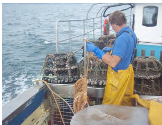
Figures 3: Attaching the pots to the ground rope whilst shooting.
