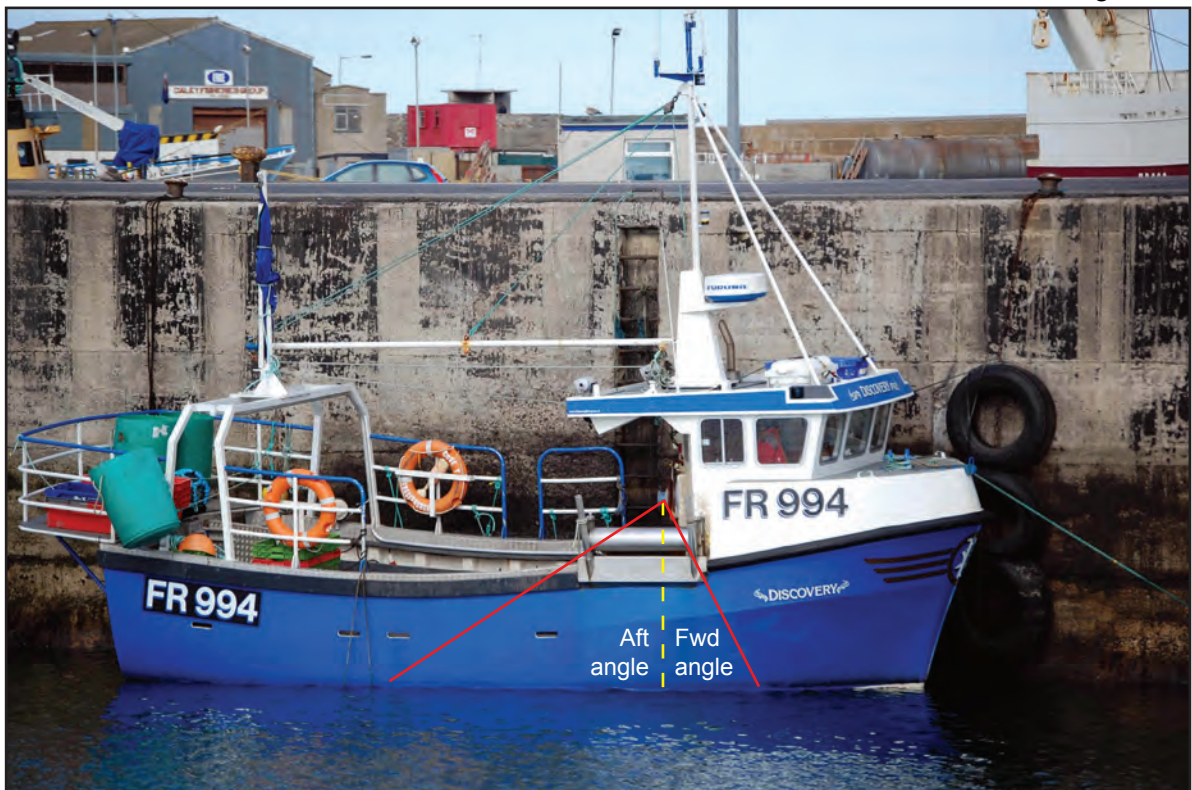
Alignment of 'V' wheel hauler onto bulwark roller
