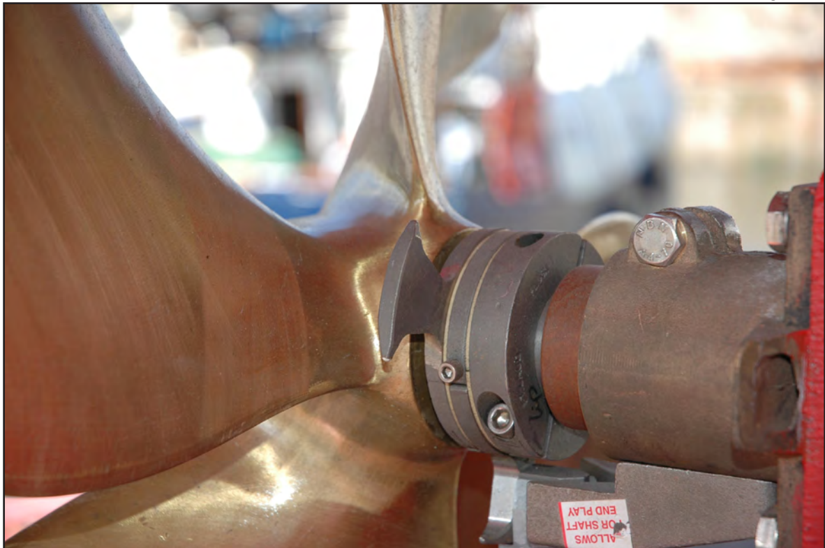
Rope cutter fitted to the propeller shaft arrangement
