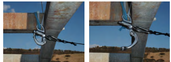
Figure 10: End weight quick release system
